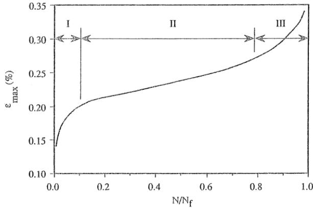
**Fig. 7. Monoaxial cycles compression test  $\sigma$ - $\varepsilon$  curve**
