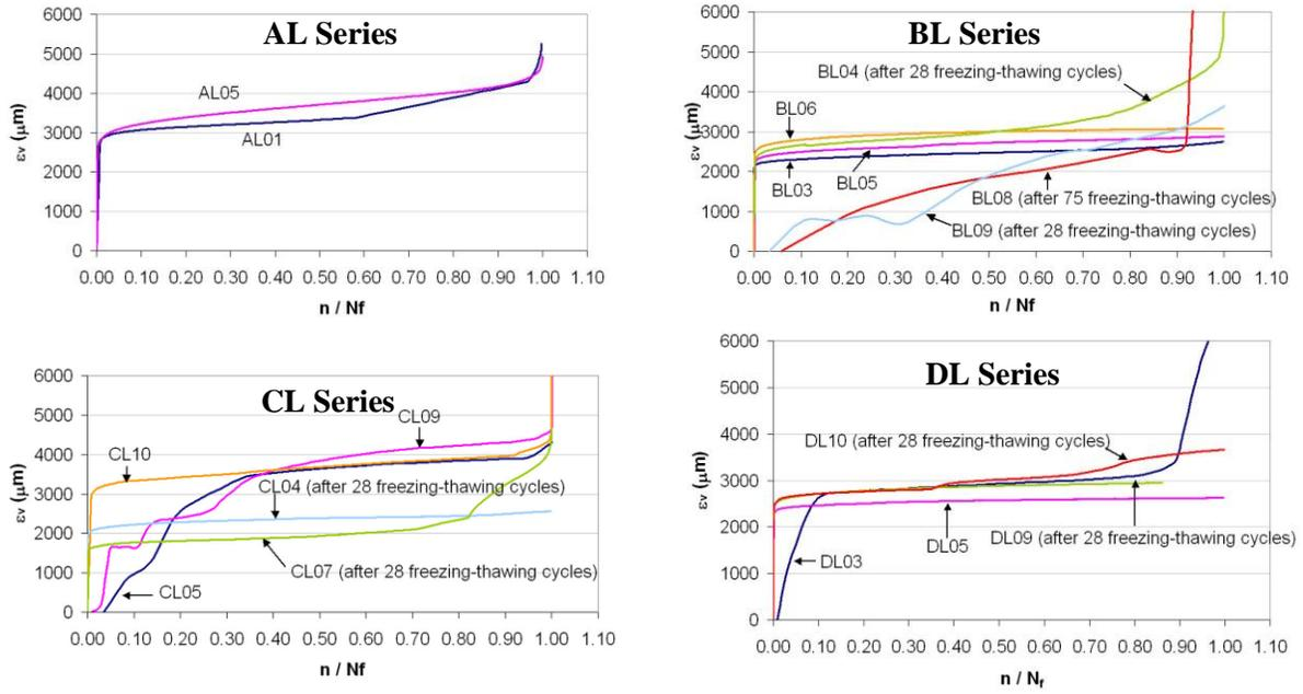
**Fig. 8. Series cyclic tests: max vertical deformation**
