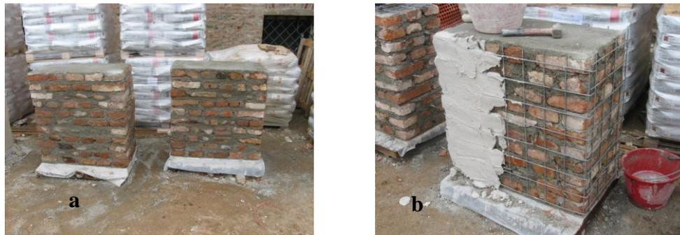
**Fig. 4. a) Two specimens reference of the historical masonry (MA) – b) Specimens reinforced through jacketing with still mesh  $\Phi 5\text{mm}/10 \times 10\text{cm}$  (RMA)**
