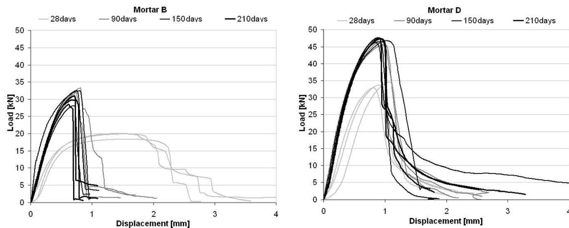
**Fig. 6. Compression test during maturation: mortar B and D**
