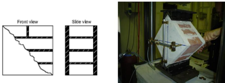
**Fig. 3. Details of the reinforced specimens and shear loading test**
