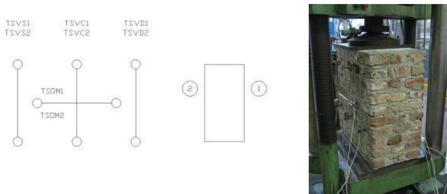
**Fig. 5. Position of transducers**
