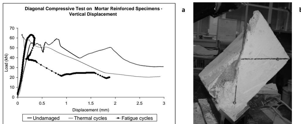
**Fig. 10. a) Diagonal compressive test on MR specimens after thermal and fatigue damage and in undamaged condition – b) MM02 specimen after collapse.**
