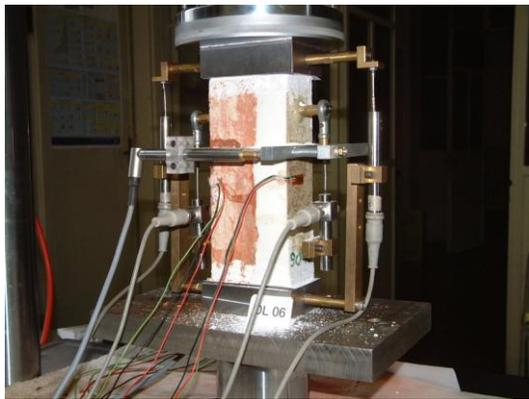
**Fig. 2. Instrumentation for mixed brick-mortar test pieces**
