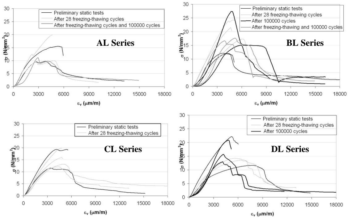
**Fig. 9. Series static tests**
