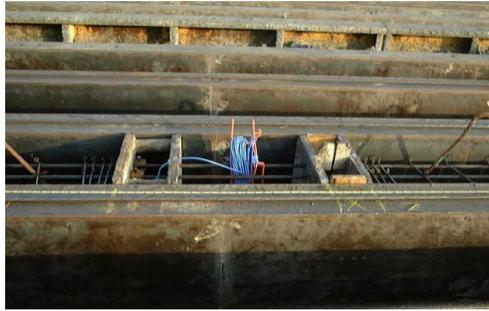
**FIGURE 3 Thermocouple Wires for Concrete Piles**
