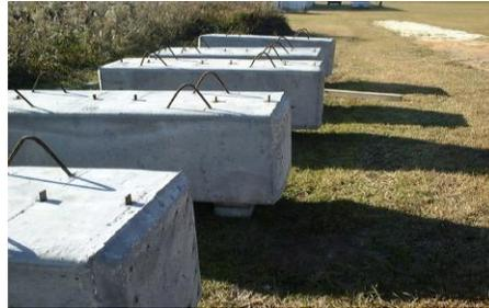
**FIGURE 6 Piles with Embedded Metal Plates**
