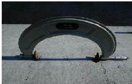
**FIGURE 7 Micrometer Measurement of Embedded Plate Distance**
