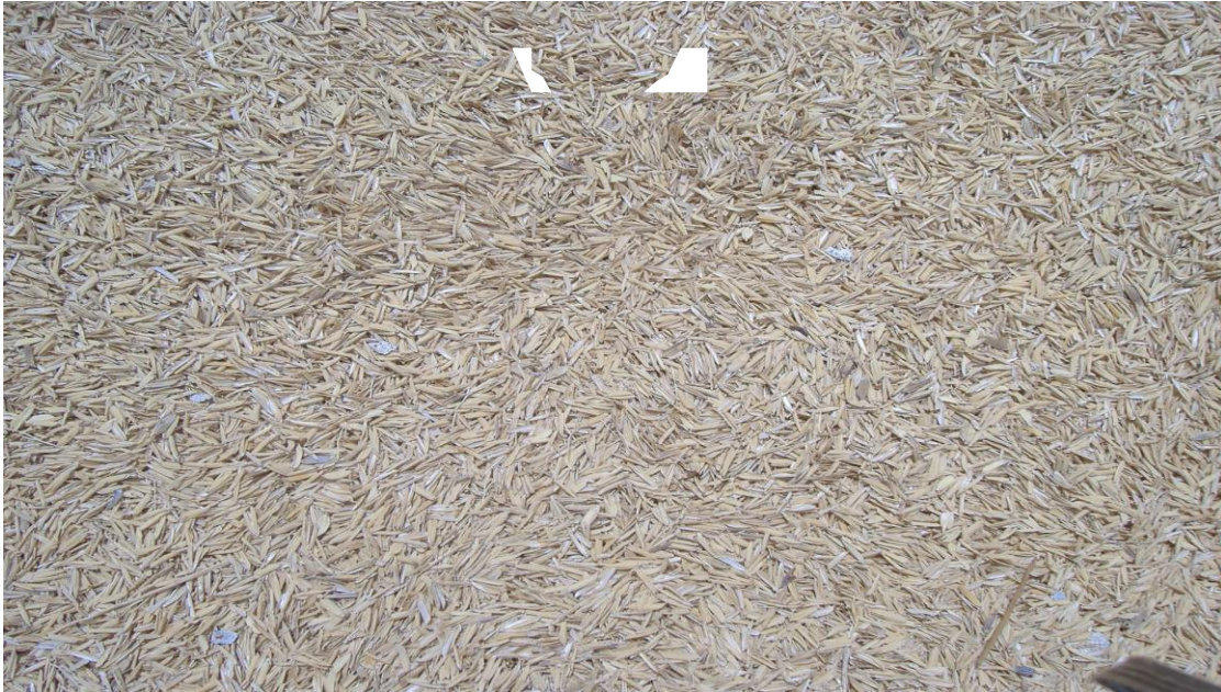
Fig. 2 Rice husk for the firing of the clay pellets.
