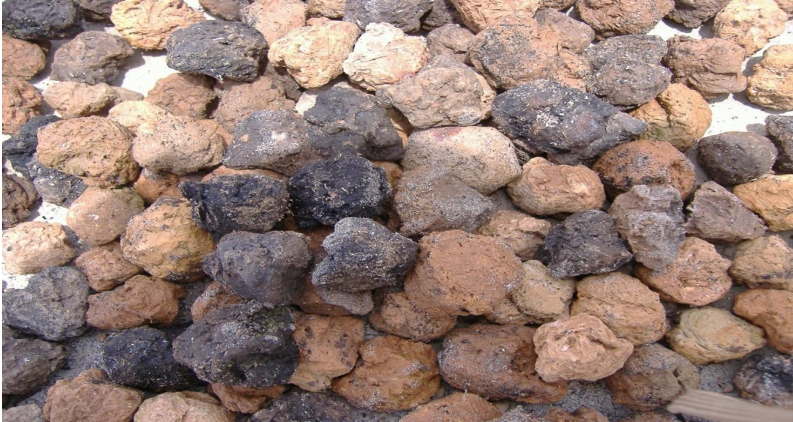
Fig. 3. Typical clay pellets resulting from the firing process.
