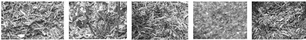
Fig. 1. to 5. From the top left corner: wood particles, grounded untreated hemp fibers and grounded and treated hemp of various fraction and from different processing centers.
