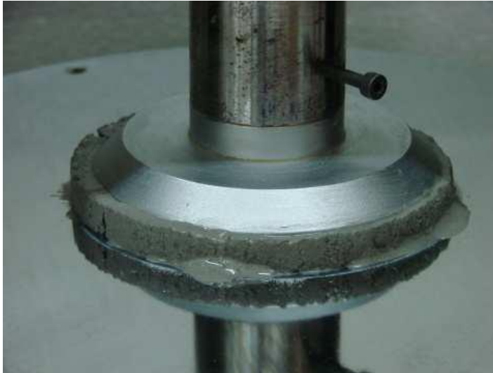
Fig. 1. Mortar workability characterization using Squeeze-flow
