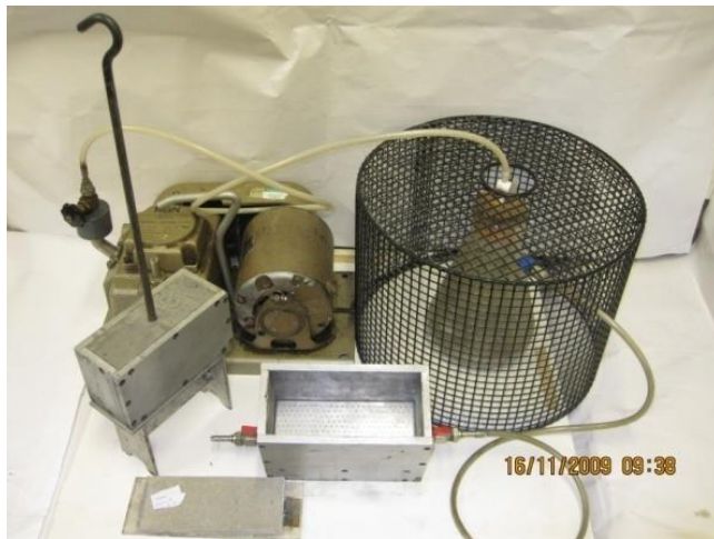
Fig. 1: Mould and a Slurry Vacuum De-watering Process Set-up.
