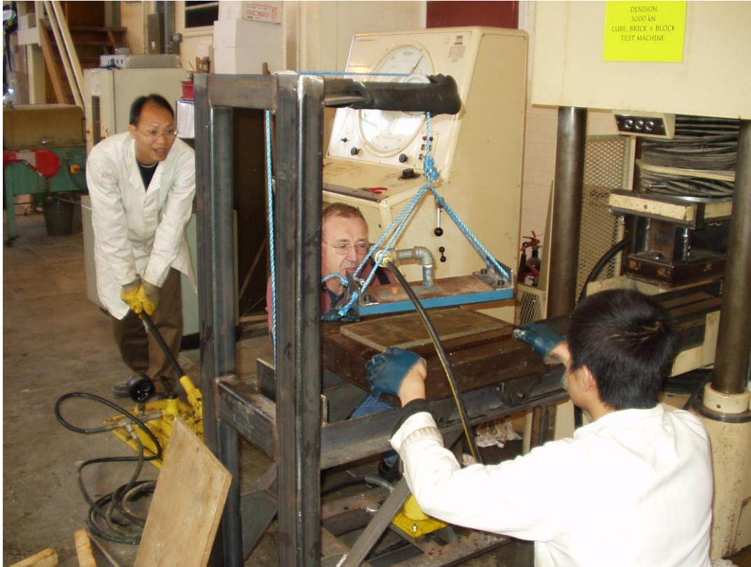
Fig. 2. Modified Compression Testing Machine for Making Concrete Paving Flags
