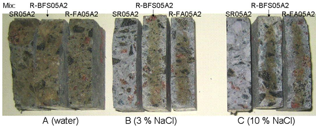
**Fig. 5. Chloride Penetration of 3 Different Mixtures After 17 cycles at Different NaCl Concentrations of 0, 3 and 10%**
