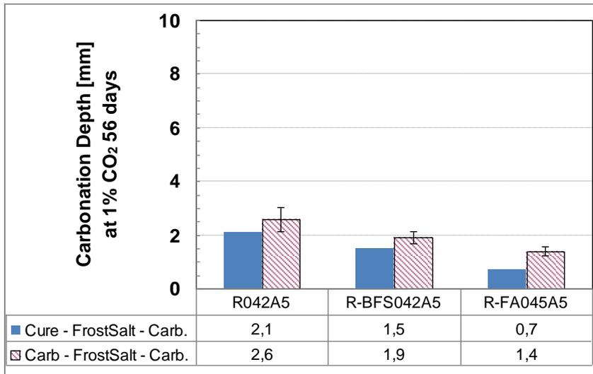
**Fig. 4. Variation in Carbonation After Frost-Salt Exposure, for 50% Slag or 24% Fly Ash**
