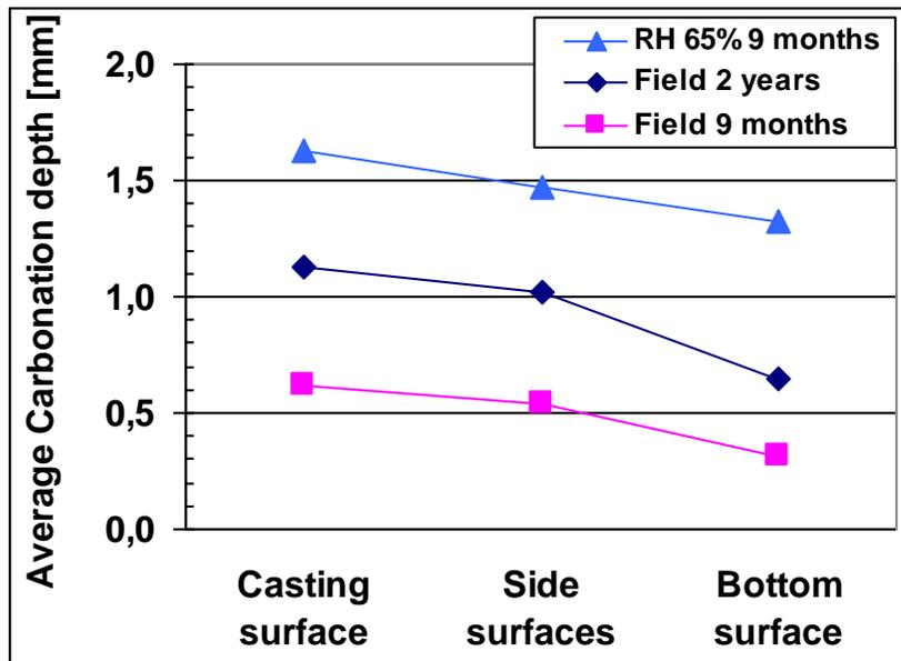
**Fig. 8. Influence of Test Surface Direction on Carbonation Depth, Average of 23 Different Mixtures**
