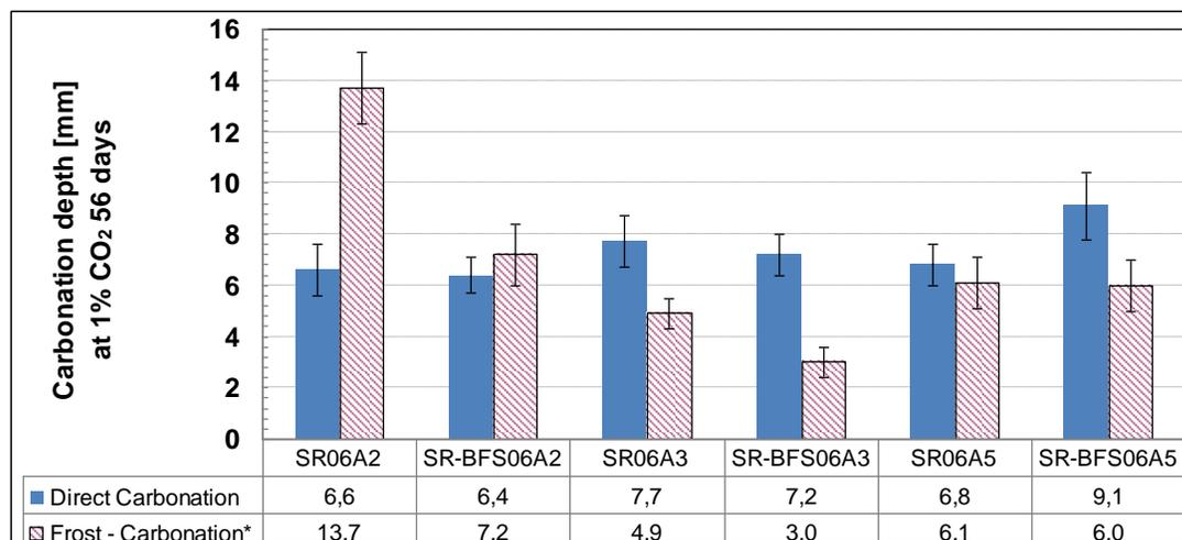
**Fig. 2. Variation in Carbonation After Frost Exposure, for 50% Slag Mixture with Changing Air Contents**
