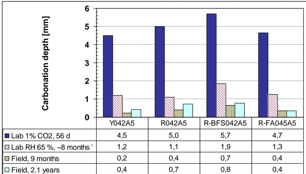
**Fig. 7. Comparison of Field and Laboratory Carbonation Measurements**
