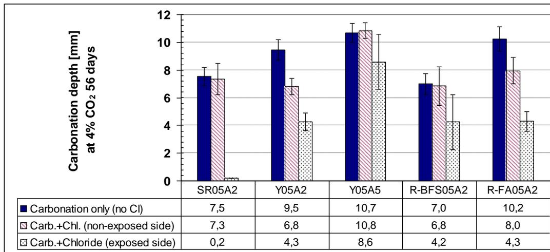
**Fig. 6. Influence of Chloride Ingress on Carbonation Depth**
