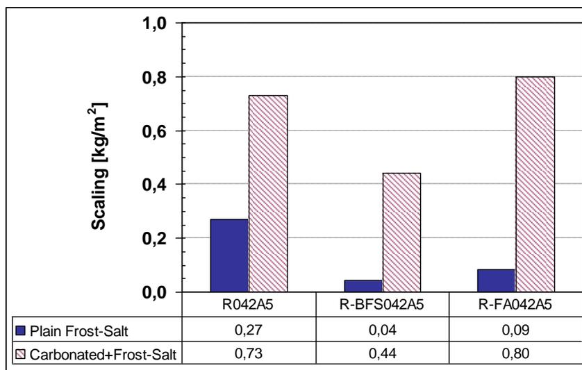
**Fig. 3. Influence of Carbonation on Scaling from Frost-Salt Testing, for 50% Slag or 24% Fly Ash Mixtures**
