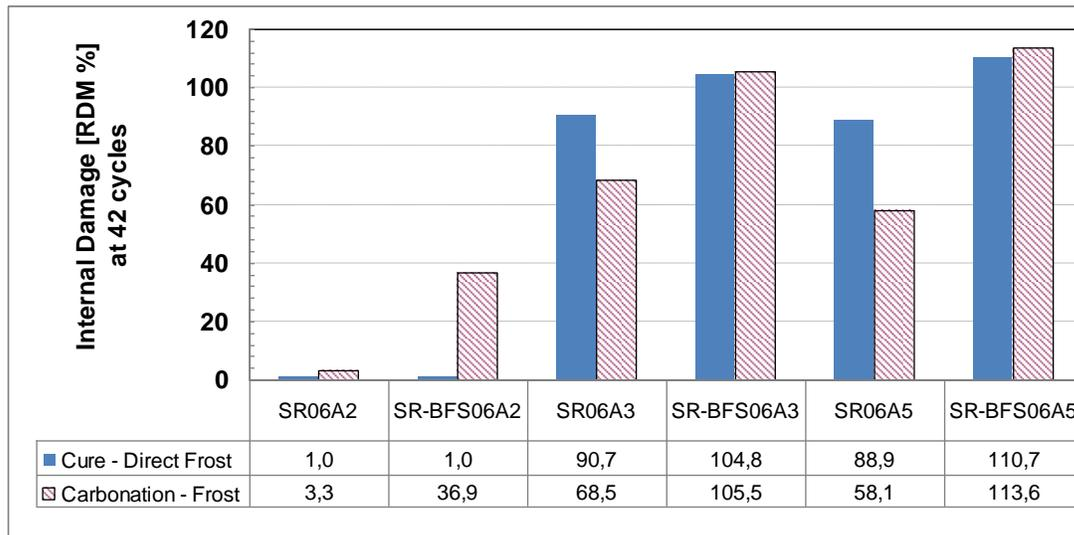
**Fig. 1. Variation in Frost Resistance (Internal Damage) After Carbonation, for 50% Slag Mixture with Changing Air Contents**
