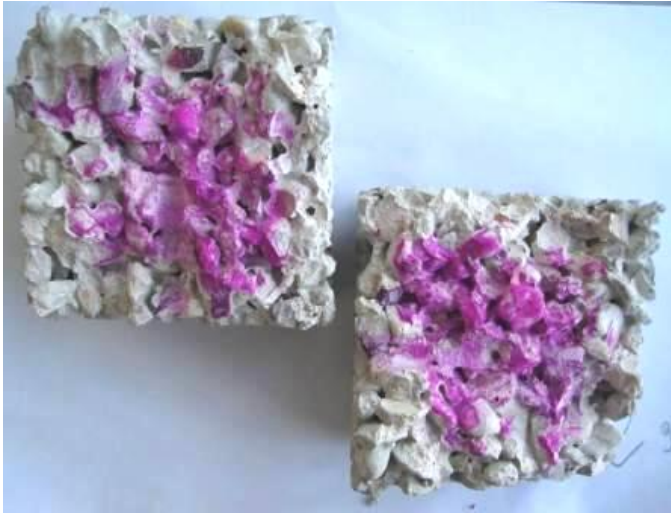
Fig. 4. Carbonation Depth of ‘RECF&c’ No-Fine Concrete after 90 Days in Atmosphere.
