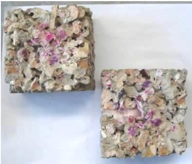
Fig. 5. Carbonation Depth of ‘RECF&c’ No-Fine Concrete after 3 Days in Climatic Chamber.
