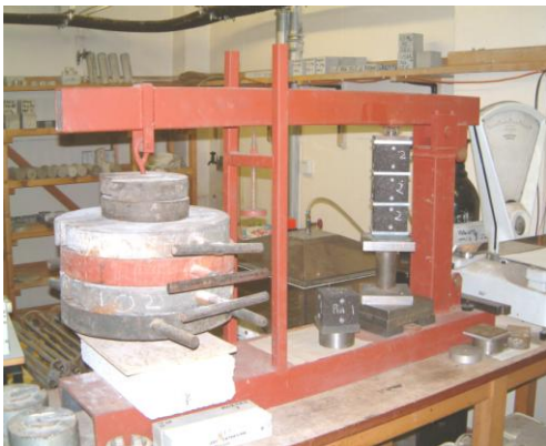
Figure 6 and 7: Static deadweight load lever arm machine and a 50mm Demec gauge with its supporting equipment.
