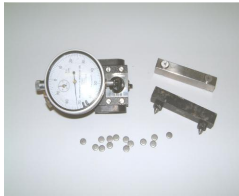
Figure 6 and 7: Static deadweight load lever arm machine and a 50mm Demec gauge with its supporting equipment.
