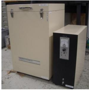
**Photo 2. Temperature-controlled chamber**
