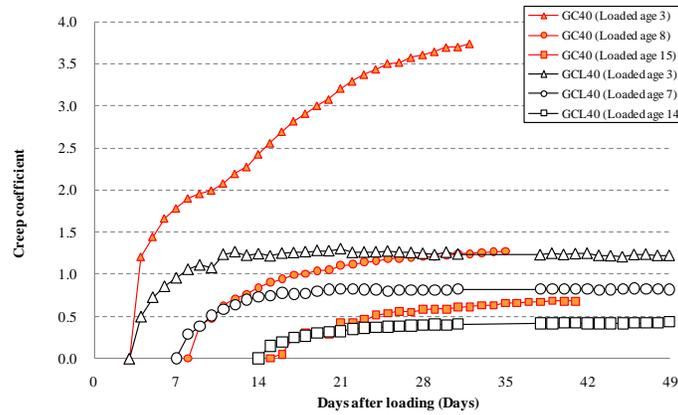
**Fig. 6. Creep coefficient (GL and GCL)**
