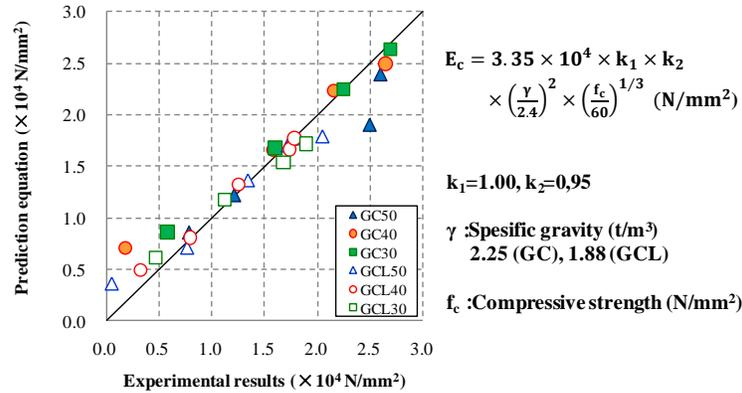
**Fig. 4. Relationship between experimental results and calculated results**
