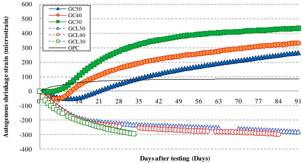
**Fig. 9. Autogenous shrinkage strain**
