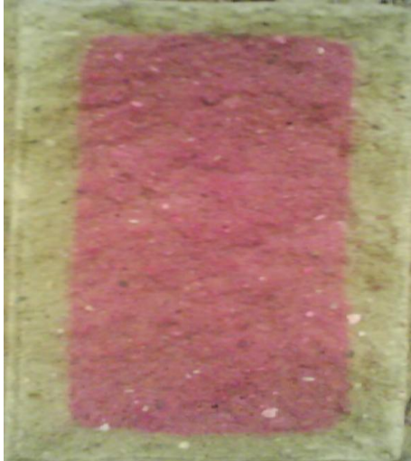
Fig. 2. 28-Day Carbonation Depth of CLSM
