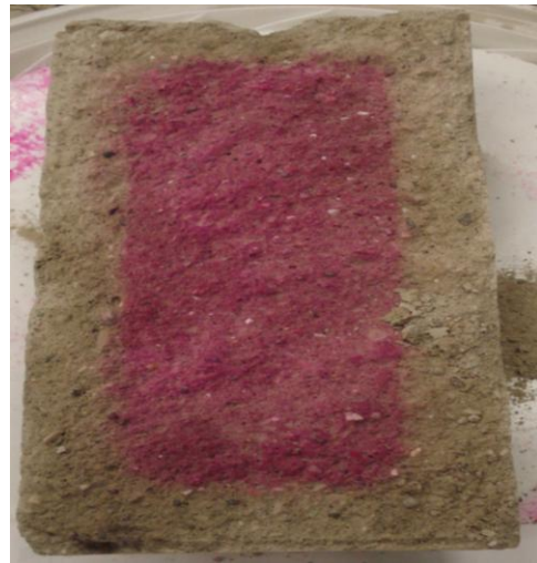
Fig. 3. 56-Day Carbonation Depth of CLSM
