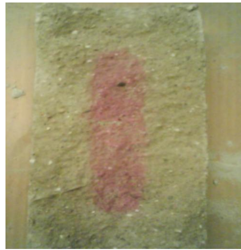
Fig. 5. 91-Day Carbonation Depth of CLSM
