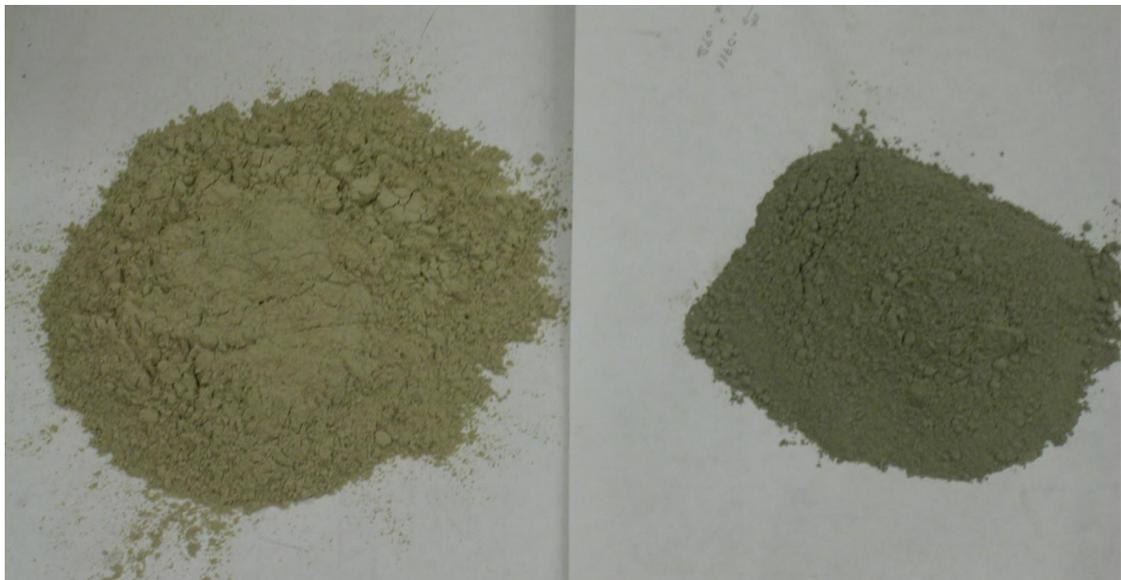
**Fig. 2. ASTM Class C Fly Ash (Left) and High-Carbon Fly Ash (Right)**
