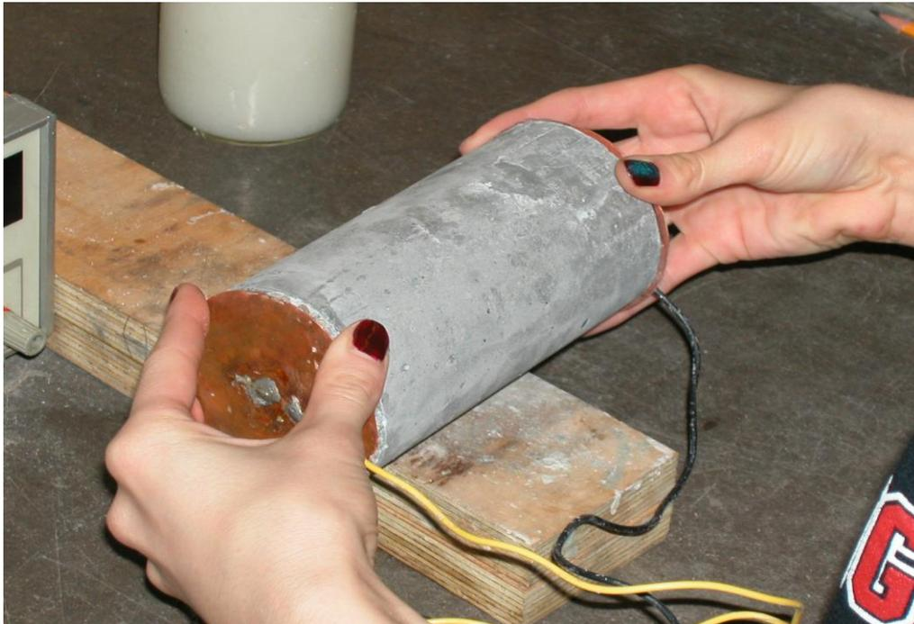
**Fig. 5. Measurement of Electrical Resistance of Concrete Test Cylinder**
