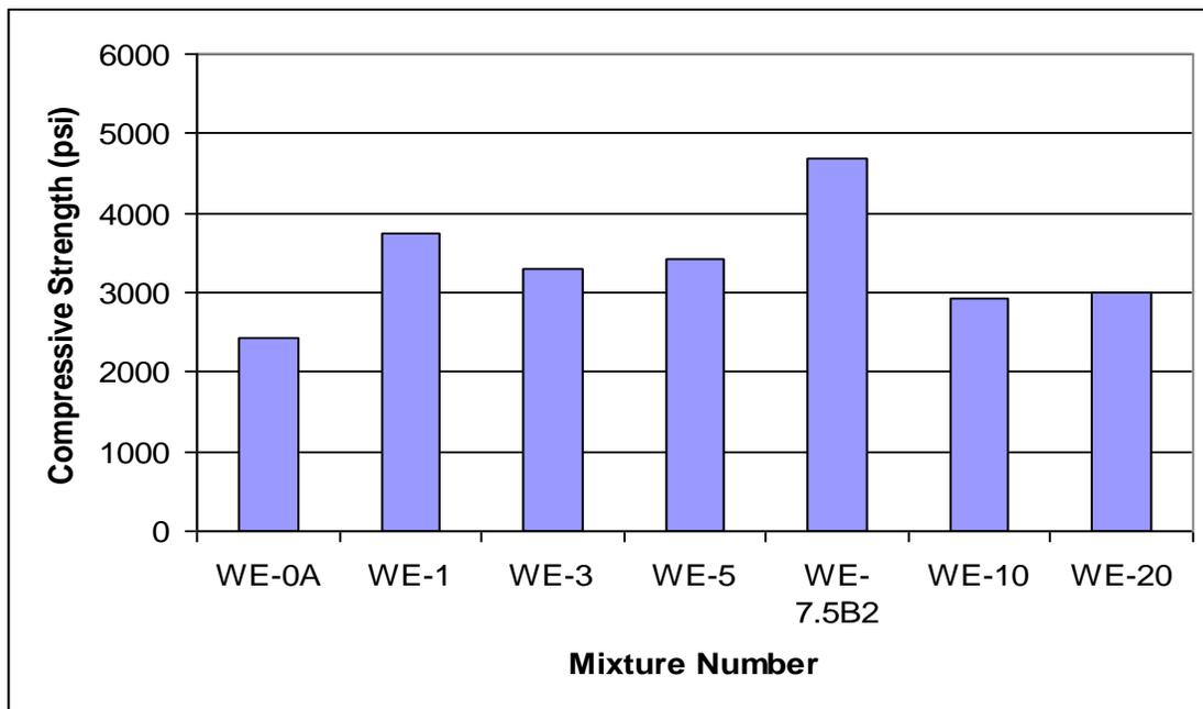
**Fig. 3. 28-Day Compressive Strength of Concrete without High-Carbon Fly Ash**
