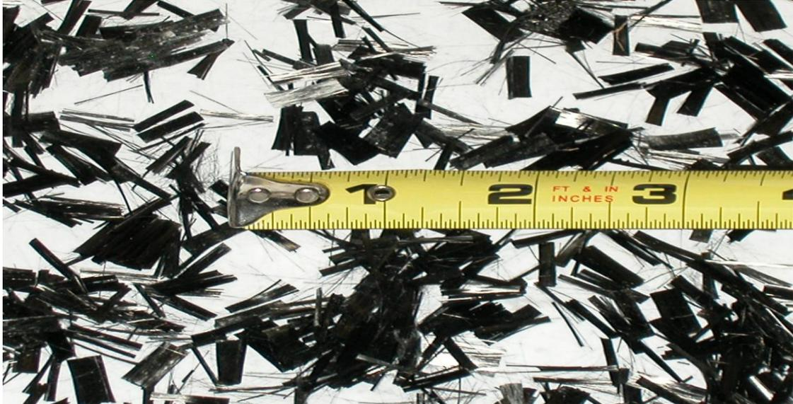
**Fig. 1. Carbon Fibers Used in Concrete Mixtures**
