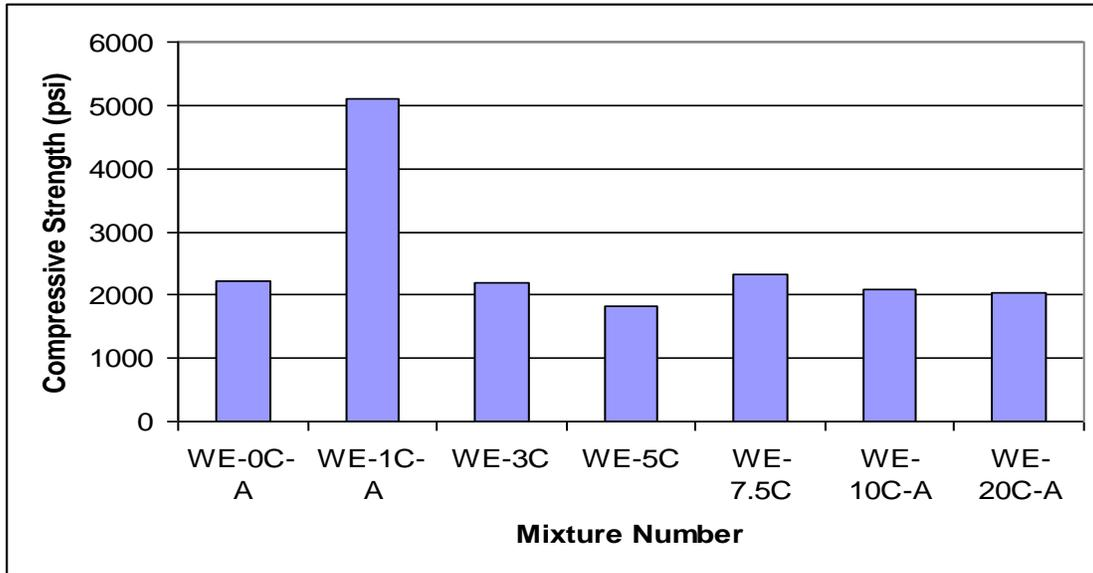
**Fig. 4. 28-Day Compressive Strength of Concrete Containing High-Carbon Fly Ash**
