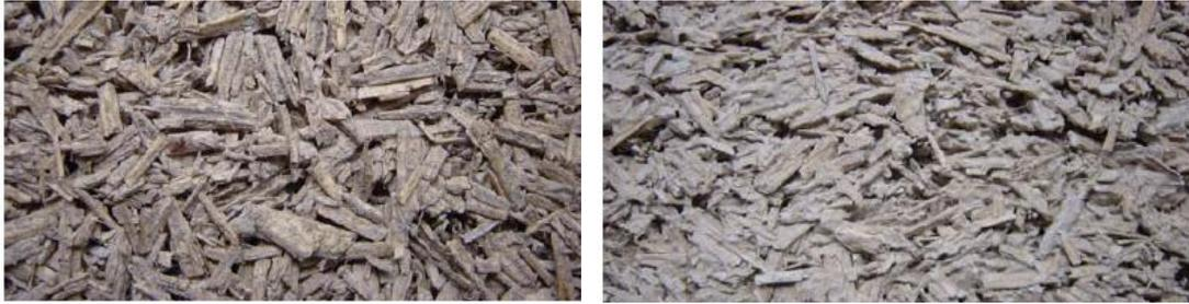
**Fig. 7. Shiv and Binder Matrix of 275 and 330kg/m<sup>3</sup> Specimens**
