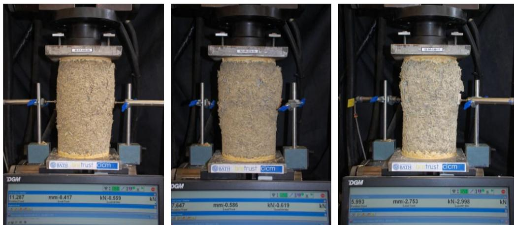
**Fig. 8. THB-B: 220, 275 and 330 kg/m<sup>3</sup> Specimens at Failure**
