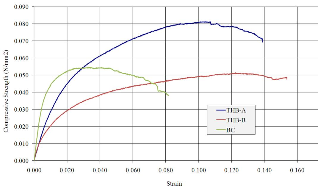
**Fig.5. 28 day Stress-Strain Relationship of Specimens Mixed with Different Binders**
