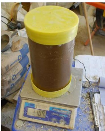
**Fig. 3. Moulded Specimen**
