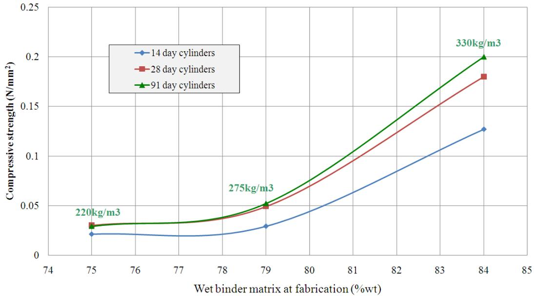
**Fig. 6. Compressive Strength vs. Wet Binder Percentage of THB-B Specimens**
