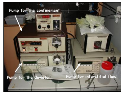
b. Three Pumps Gilson
