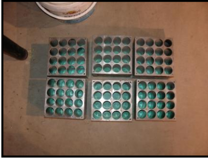
Fig. 2. Moulds Used for Obtaining Samples of (Ø36, H=100) mm
