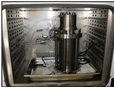
c. Triaxial Cell in the Oven
