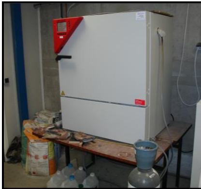
Fig.3. Climatic Chamber Attached with a Bottle of CO 2
