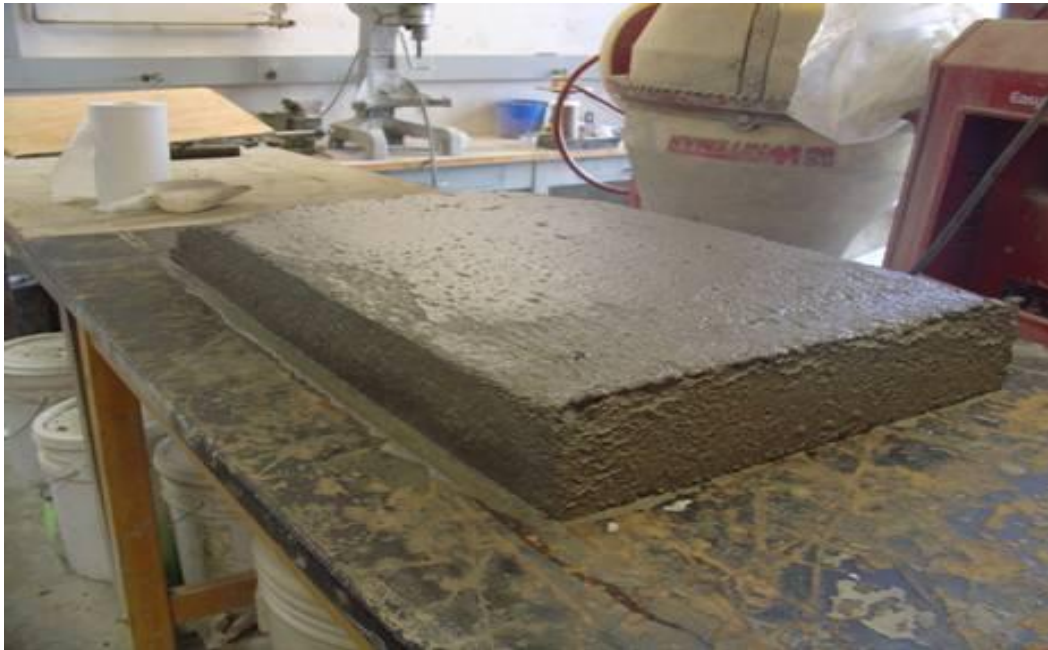
Fig. 4. Pavement containing fly ash and clay produced without vibration.
