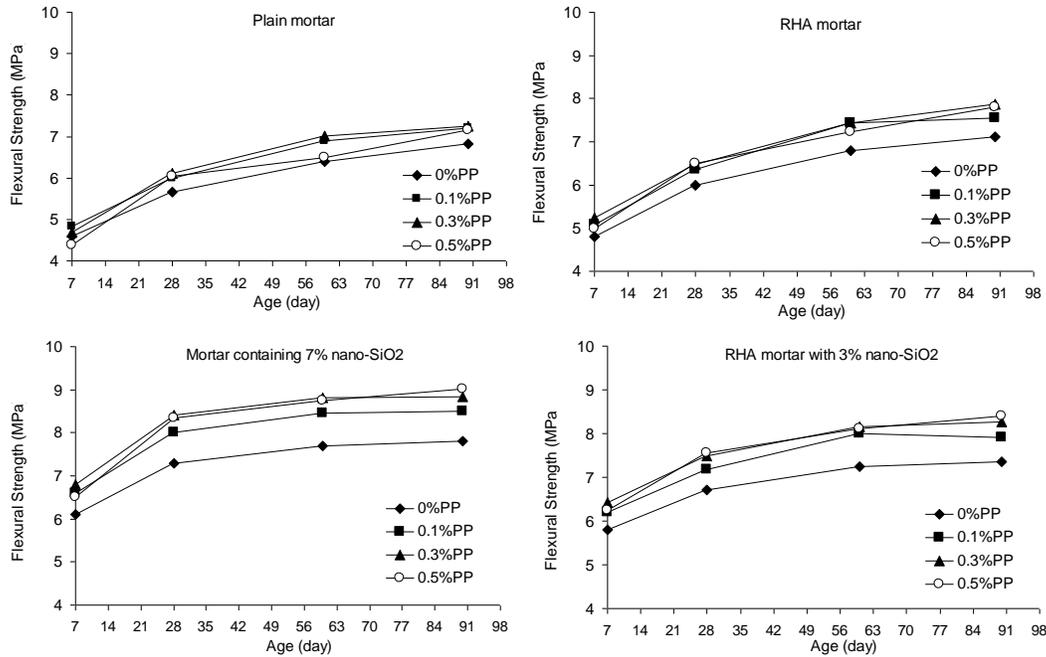
**Fig. 4. Flexural Strength of Different Mortars According to the PP Content**
