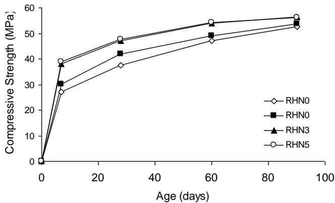
**Fig.2. Compressive Strength of RHA Mortars at Different Contents of Nano-SiO<sub>2</sub>**
