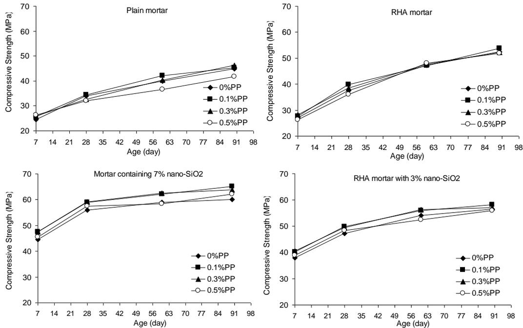
**Fig. 3. Compressive Strength of Different Mortars According to the PP Content**
