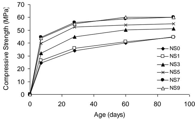
**Fig.1. Compressive Strength of Plain Mortars at Different Contents of Nano-SiO<sub>2</sub>**
