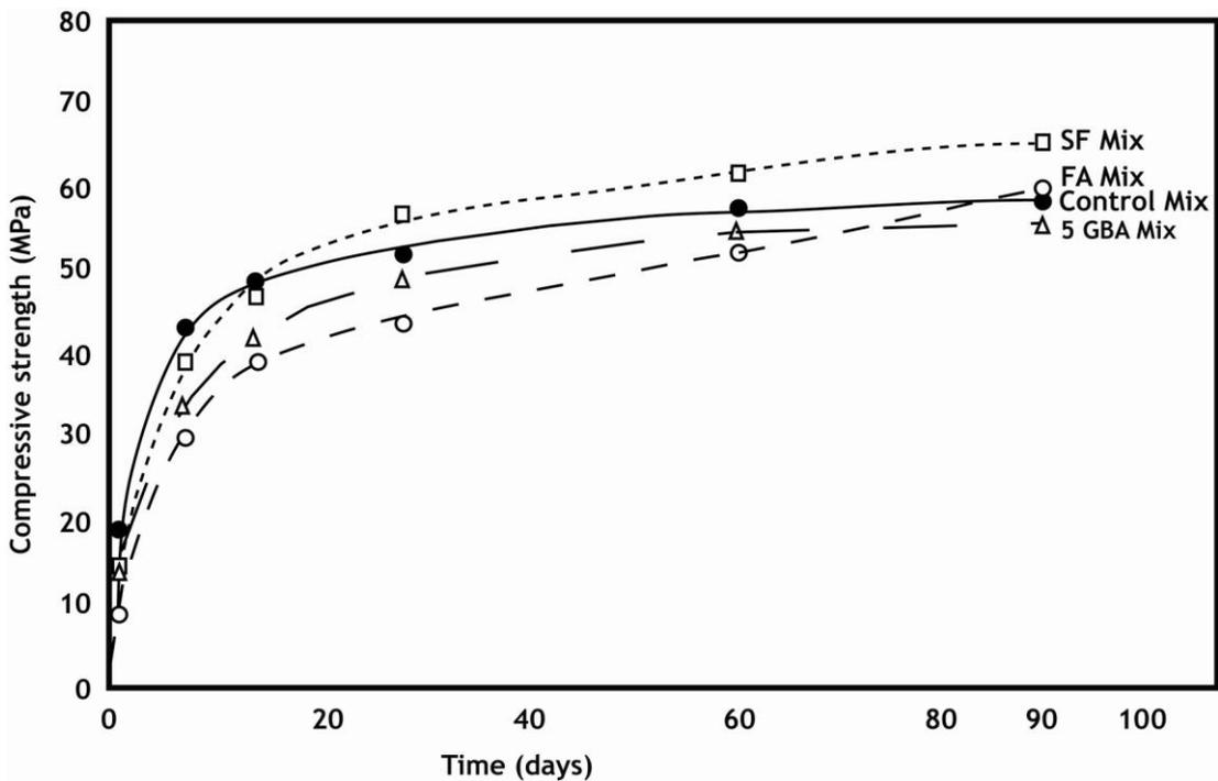
Fig. 3. Compressive strength of concrete with 5- $\mu$ m ground bottom ash (5 GBA), fly ash (FA) and silica fume (SF).
