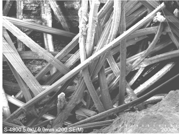
Fig 12. Magnified Image showing Striated Needles of Dicalcium Aluminate Hydrate (C 2 AH 8 )
