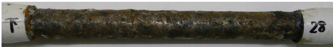
Fig. 3. Corrosion Products on a Steel Bar after Anodic Dissolution Treatment in the Concrete
