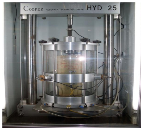
Figure 2. Triaxial Sample with LVDT's Mounted
