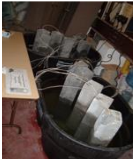
Fig. 3. Specimens in accelerated corrosion tidal cycle tanks
