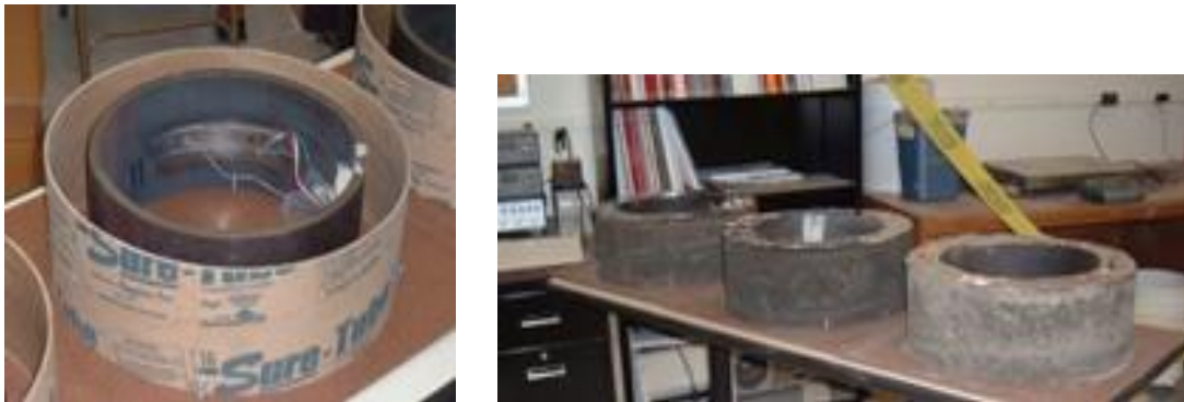
Fig. 1. Restrained shrinkage specimens
