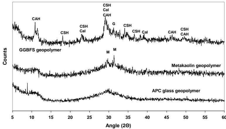
CSH - Calcium silicate hydrate, Cal - Calcite, CAH - Calcium aluminium oxide hydrate, M - Muscovite, G - Gypsum
