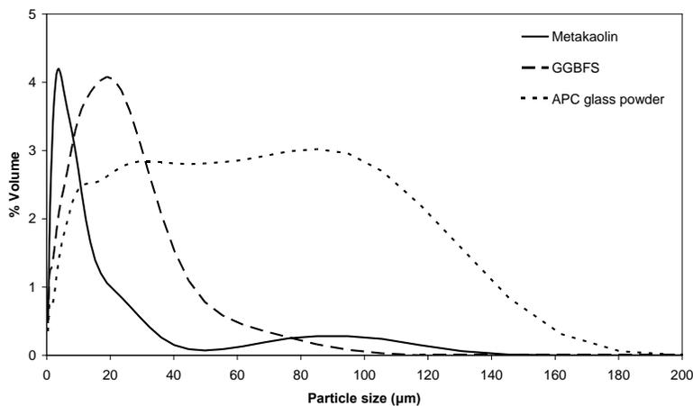
**Fig. 1. Particle Size Distribution of APC Glass, Metakaolin and GGBFS**
