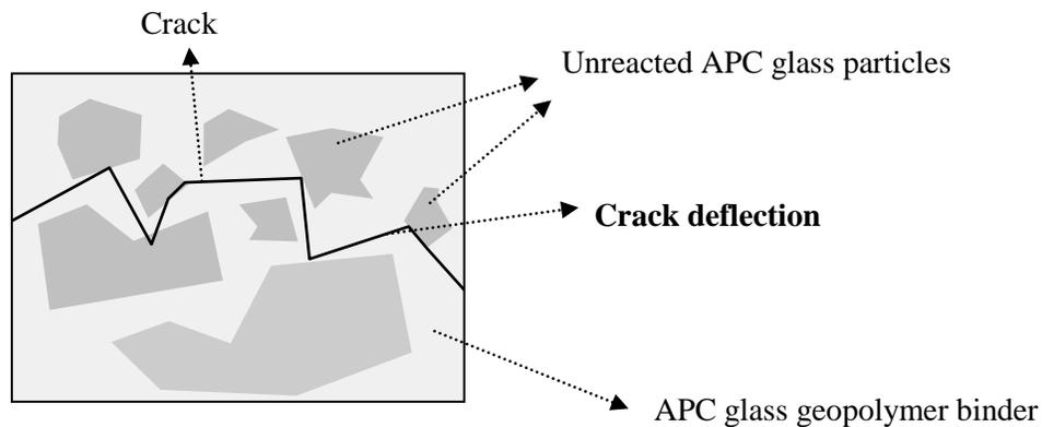
**Fig. 7. Schematic Diagram Showing the Crack Deflection Mechanism in APC Glass Geopolymers**
