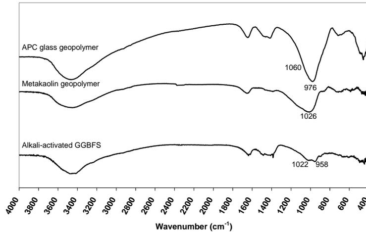
**Fig. 6. FTIR Analysis of APC Glass, Metakaolin and GGBFS Geopolymers**
