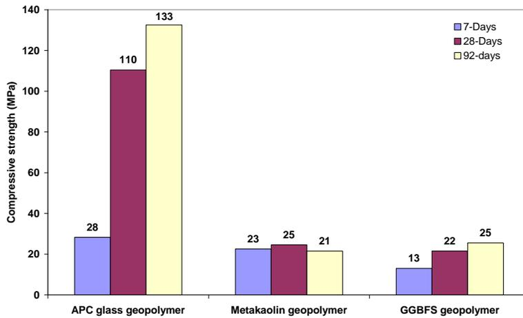
**Fig. 3. Compressive Strength Data at 7 28 and 92 Days for APC Glass, Metakaolin and GGBFS Geopolymers**
