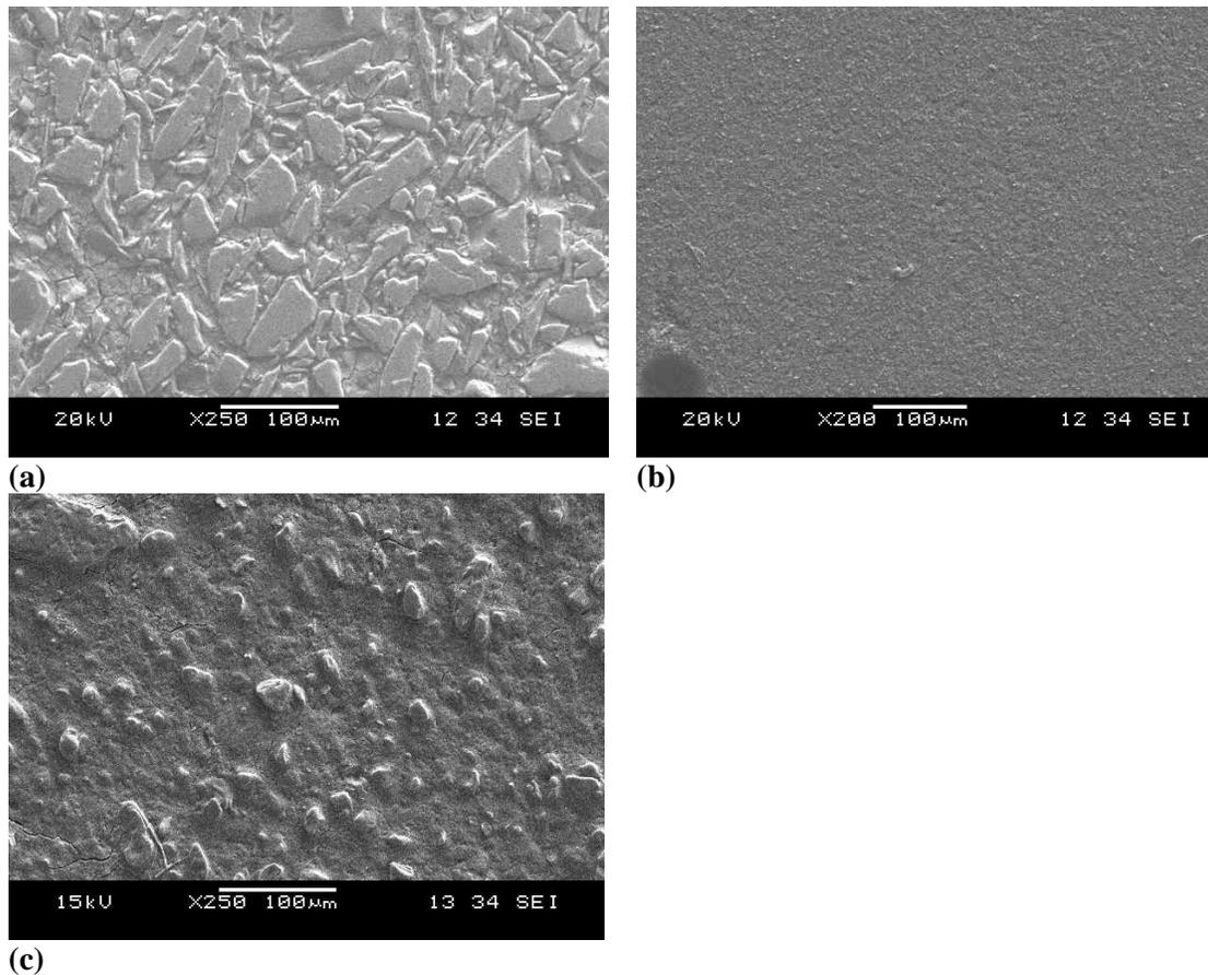
**Fig. 5. SEM Images Showing the Microstructure of: (a) APC Glass Geopolymer, (b) Metakaolin Geopolymer, (c) GGBFS Geopolymer**
