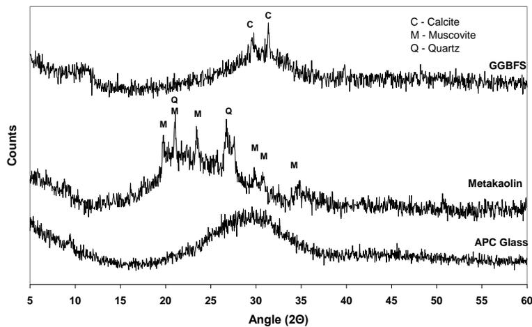
**Fig. 2. XRD Analysis of APC Glass, Metakaolin and GGBFS**
