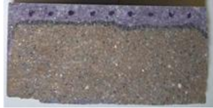
Fig. 1: Sample Prepared with CEM II after 90 Days Hardening at 100% RH, and After the Chloride Forced Migration Test. The White part Corresponds to the Region where Chlorides have Penetrated Due to the Electric Field Applied, while the Rest of the Sample has not Suffered Chloride Ingress.
