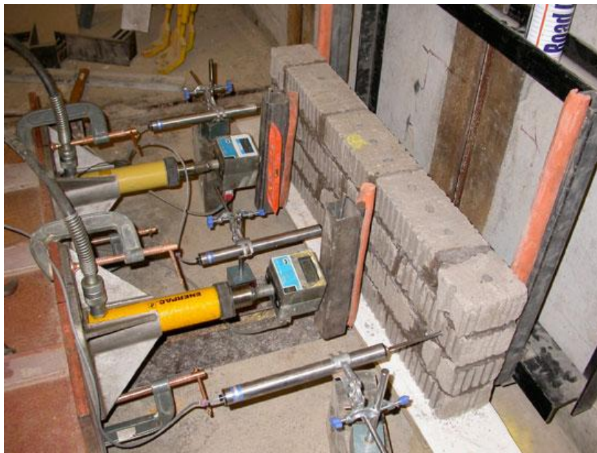
Fig. 7: Set-up for Flexural Tests (Vertical) according to BS EN 1052-2:1999
