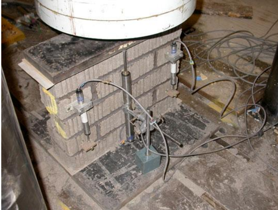
Fig. 6: Set-up for Compressive Tests according to BS EN 1052-1:1999
