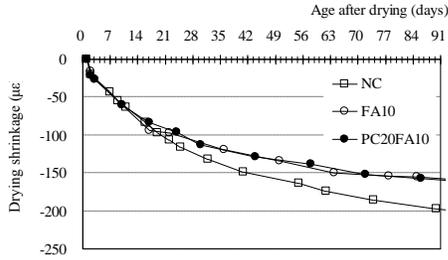
**Fig.9. Drying Shrinkage Strain, W/B=0.50**
