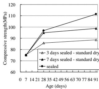
**Fig.7.Effect of the Age at Exposure to Drying on Compressive Strength Development of PC20FA20 (W/B=0.30)**
