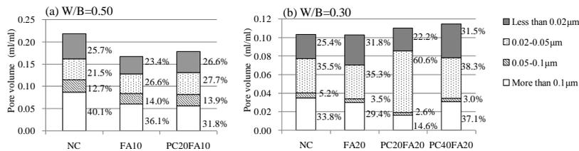
**Fig.8.Pore Size Distribution (Under Sealed Conditions)**
