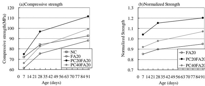
**Fig.5. Effect of Replacement Ratio of Porous Ceramic Waste on Compressive Strength of Sealed FA20 Concrete (W/B=0.30)**
