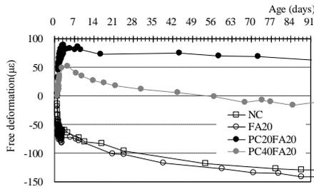
**Fig.10. Autogenous Shrinkage Strain, W/B=0.30**
