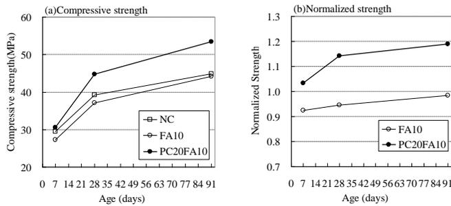
**Fig.3.Effect of Internal Curing by Porous Ceramic Waste Aggregate on Compressive Strength of Sealed FA10 Concrete (W/B=0.50)**
