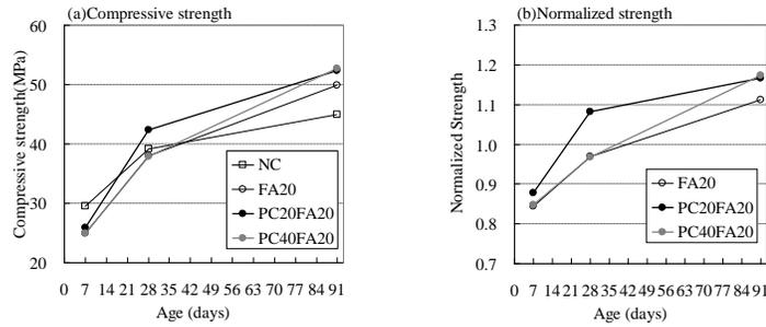
**Fig.4. Effect of Replacement Ratio of Porous Ceramic Waste on Compressive Strength of Sealed FA20 Concrete (W/B=0.50)**
