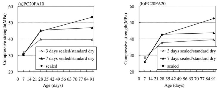
**Fig.6.Effect of the Age at Exposure to Drying on Compressive Strength Development of PC20FA10 and PC20FA20 (W/B=0.50)**
