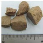
**Fig.1. Porous ceramic Coarse aggregates (PCA)**
