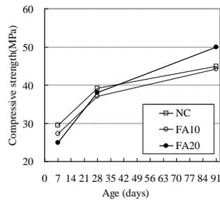
**Fig.2. Influence of Replacement Ratio of FA on Compressive Strength of Sealed Concrete (W/B=0.50)**
