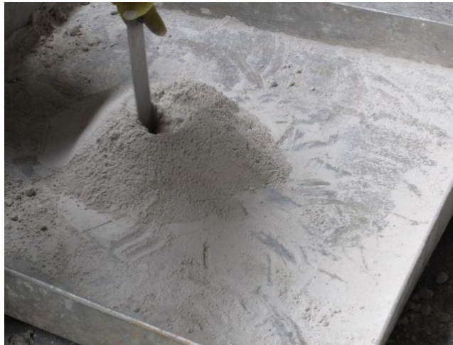
Fig 5. Mixing of Kaolin with optimum moisture content
