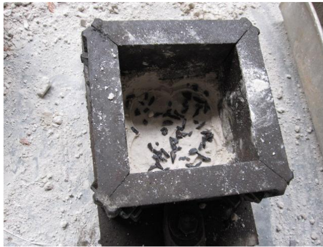
Fig7.View of 1/3 Layer with Shred Tire in Mould
