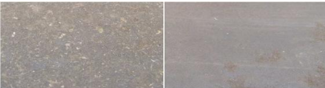
Fig. 5: on the right, a board made from the mixture 60 (fraction B cannabis); on the left, without a cement sub-base
