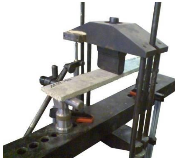
Fig. 3: The tests of modulus of elasticity and bending strength
