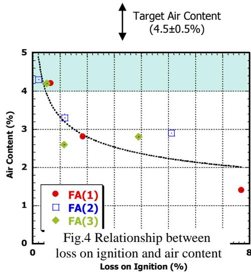
Fig.4 Relationship between loss on ignition and air content
