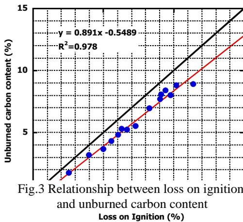
Fig.3 Relationship between loss on ignition and unburned carbon content
