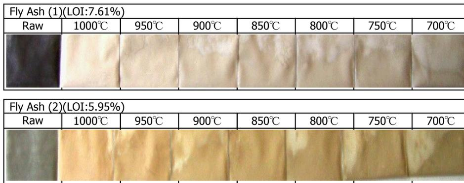
Fig. 8 Burning temperature and colour of CfFA
