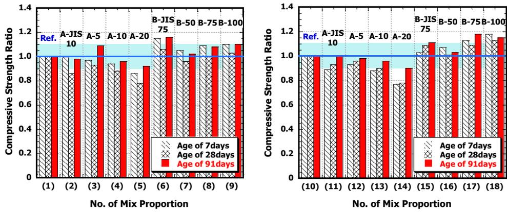
Fig.12 Compressive strength ratio of CfFA concrete
