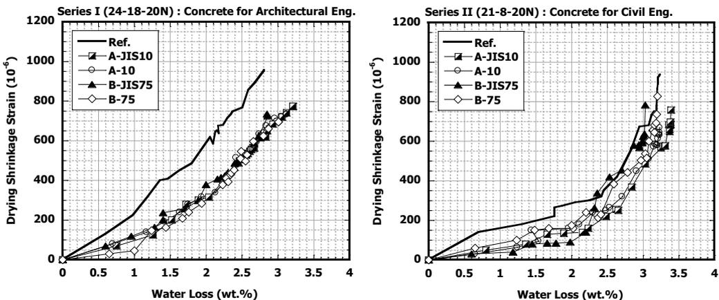
Fig.16 Relationship between water loss and drying shrinkage strain
