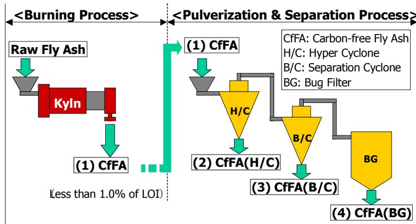
Fig.5 Outline of production system of CfFA
