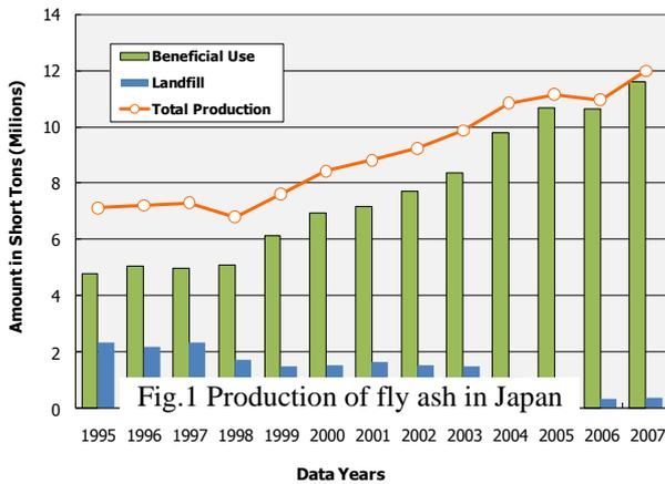
Fig.1 Production of fly ash in Japan
