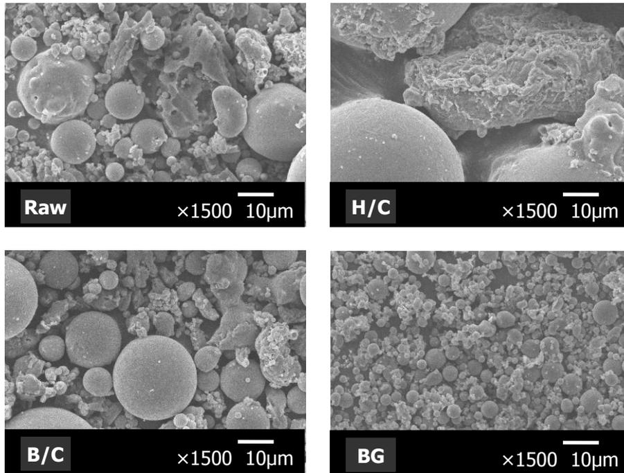
Fig. 7 SEM pictures of fly ash (Fly Ash (1))
