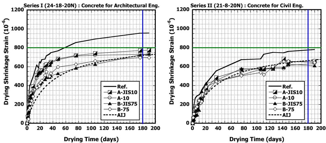
Fig.15 Drying shrinkage strain
