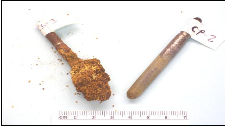
Fig. 2. Corrosion Observed on Uncoated Rod (Left) Compared to Uncorroded Vitreous-Ceramic Coated Test Rods (Right) After 40-Days Exposure to Sand Saturated with 3.5% NaCl Solution. The Dull Surface on the Uncorroded Rod was Formed when the Exterior Layer of Portland Cement Hydrated
