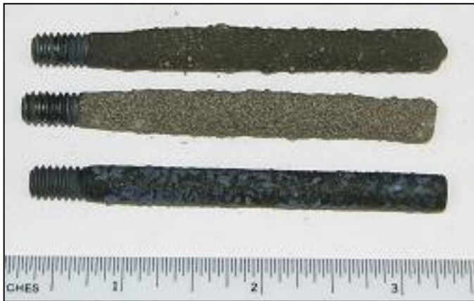
Fig. 1. Examples of Steel Test Rods Coated with Vitreous Enamel with an Outer Layer of Fused Cement. One in. = 2.54 cm.
