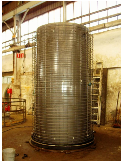
Fig. 2. Vertical casting position (inner mould)
