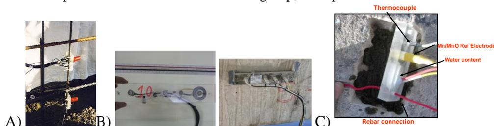
**Fig. 1. A) Embedded sensors for electrochemical measurements installed in a dock in the south of Spain. B) Surface sensors installed inside a bridge. C) Passive sensors installed in Zarzuela Racecourse.**
