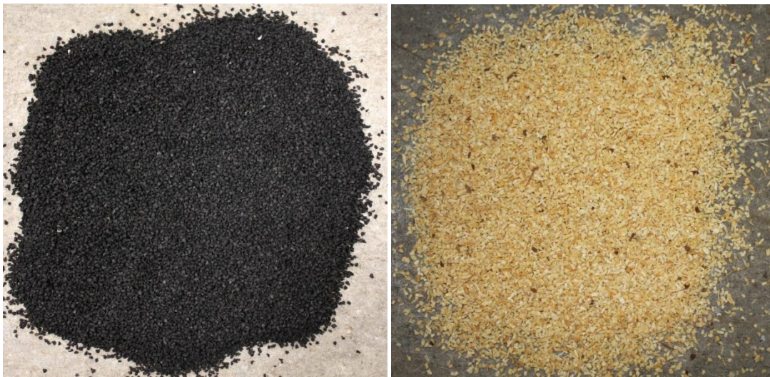
Fig. 2. Fine Aggregate Gradations of (a) Crumb Rubber and (b) Sawdust.
