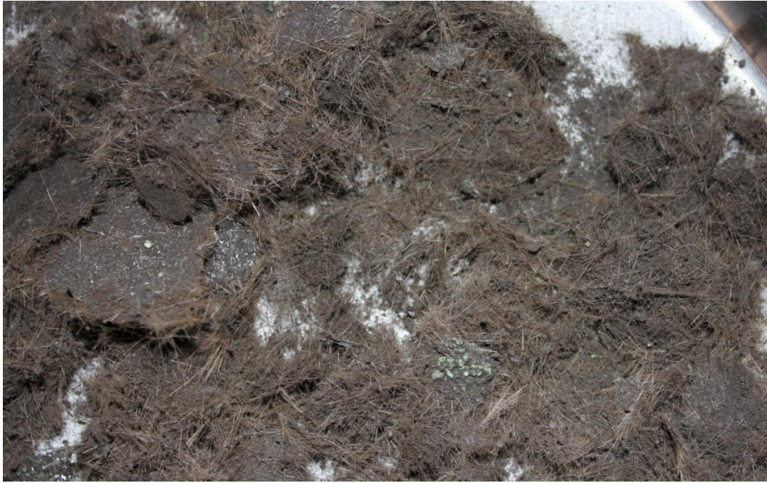
Fig. 1. Roofing Shingle Scrap after Initial Shredding.
