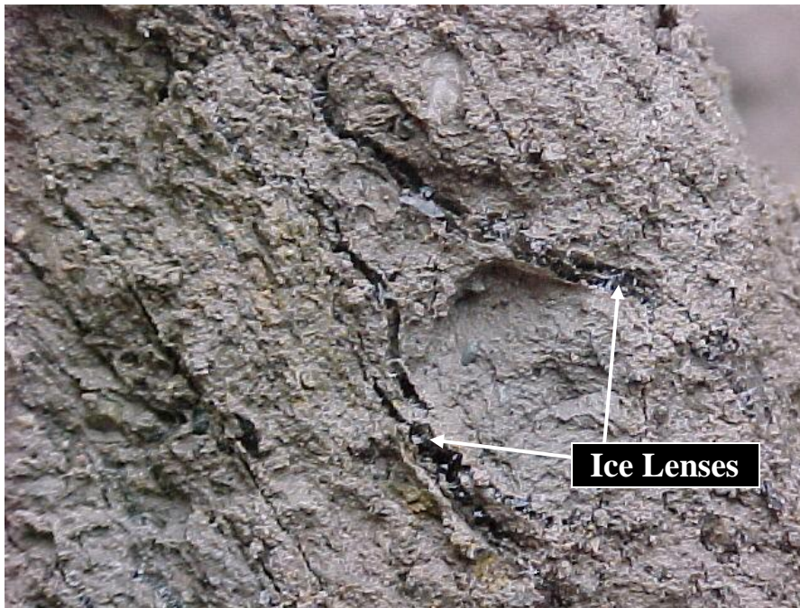
Figure 2. Ice lenses in sample taken from problem subgrade of Illinois Route 53 near Gardner, Illinois.
