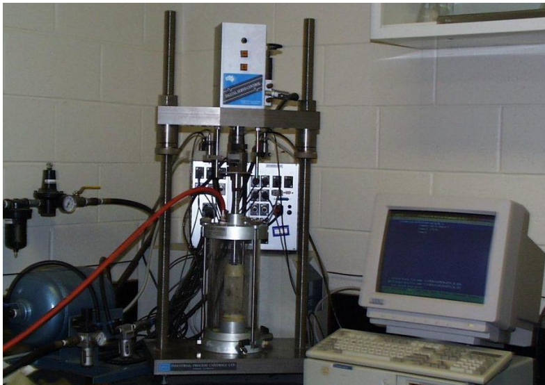
Fig. 1. Triaxial test setup for monotonic loading of the soil specimen
