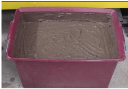
Figure 3. Remoulded soil left to cure overnight.
