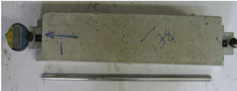
Fig. 1. Unrestrained Shrinkage Measuring Setup
