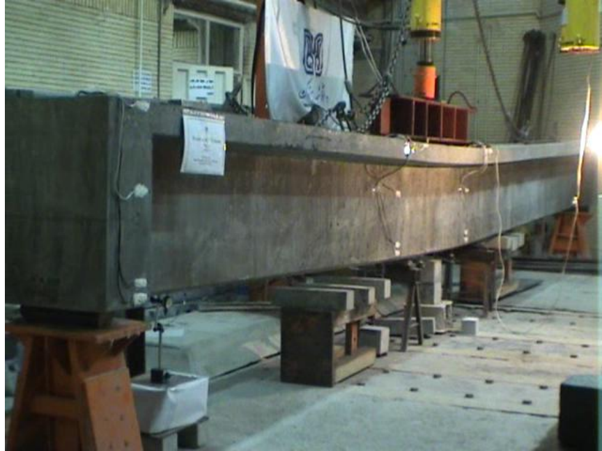
Figure 1 – Details of PSCC beams tested
