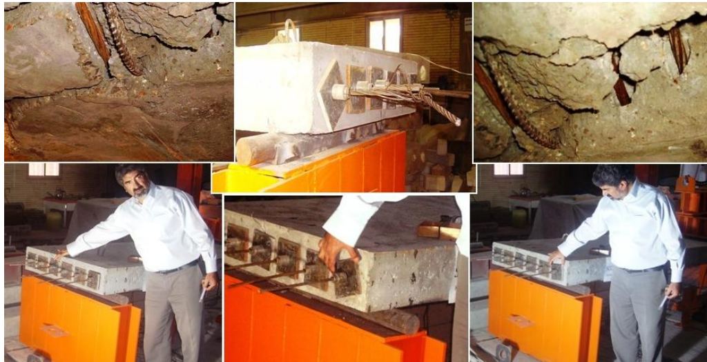
Fig. 9 – Rupture of tow tendons in SCC slab1
