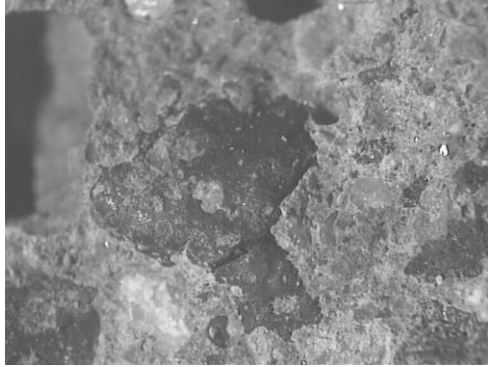
Figure 4. Good cement paste-aggregate bonding
