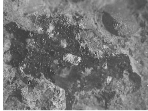
Figure 5. Salt concentration in slag aggregate
