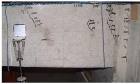
Figure 10. Concrete Cracking (after previous cyclic load)
