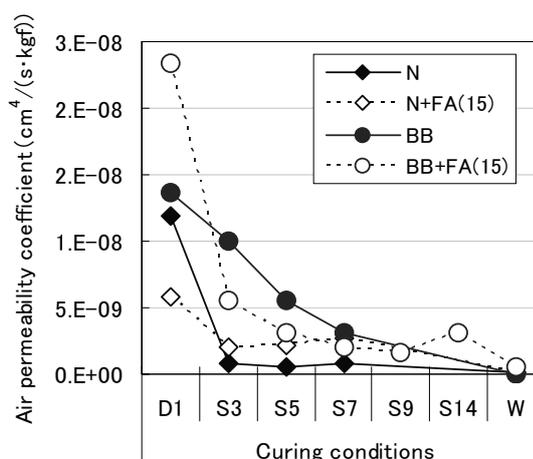
Figure 12. The relation between curing conditions and Air permeability coefficient
