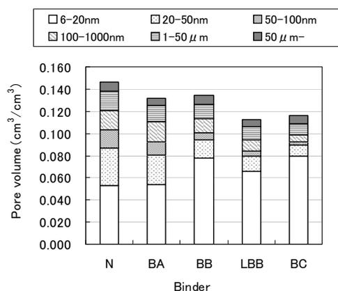
Figure 7. Micropore distribution: the central portion of concrete
