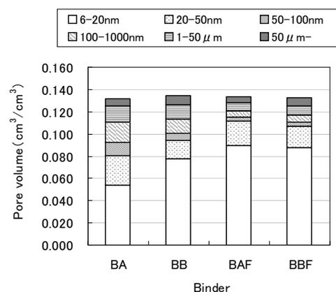
Figure 8. Micropore distribution: the central portion of concrete added FA
