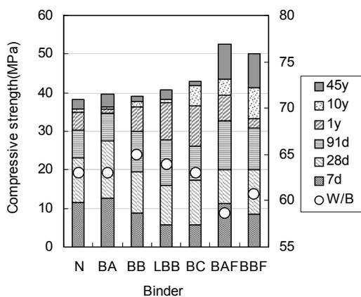
Figure 5. Compressive strength of concrete with each binder
