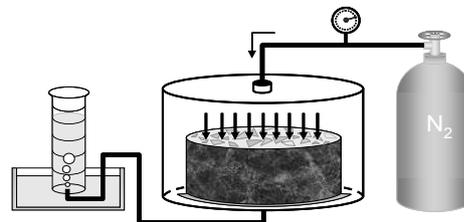
Figure 3. Gas permeability test
