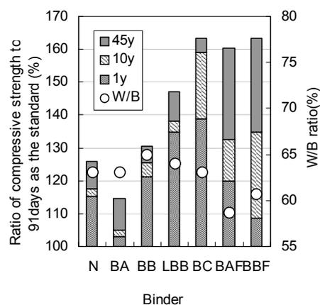
Figure 6. Ratio of compressive strength to 91 days as the standard
