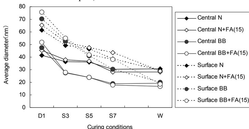
Figure 14. Effect of curing conditions on average diameter of pore
