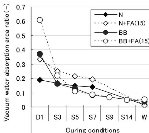
Figure 13. The relation between curing conditions and vacuum water absorption
