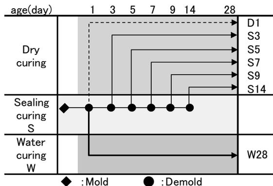
Figure 1. Curing conditions and method
