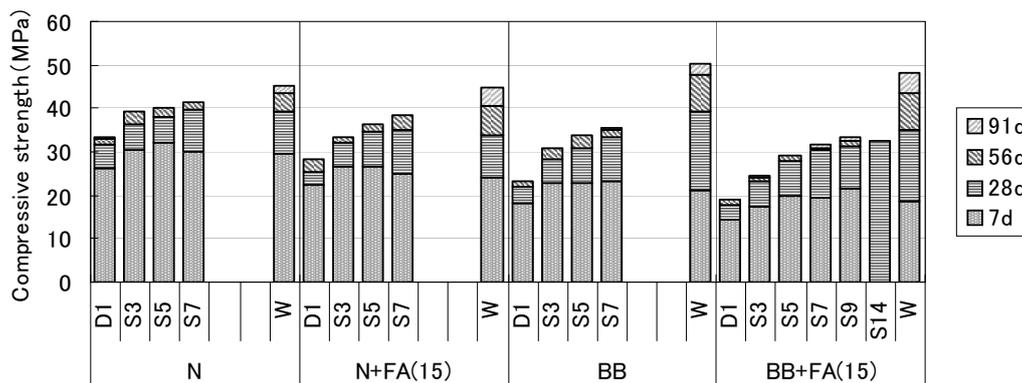
Figure 10. Compressive strength of concrete under different curing conditions
