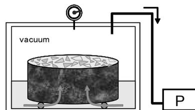
Figure 4. Water absorption test in vacuum
