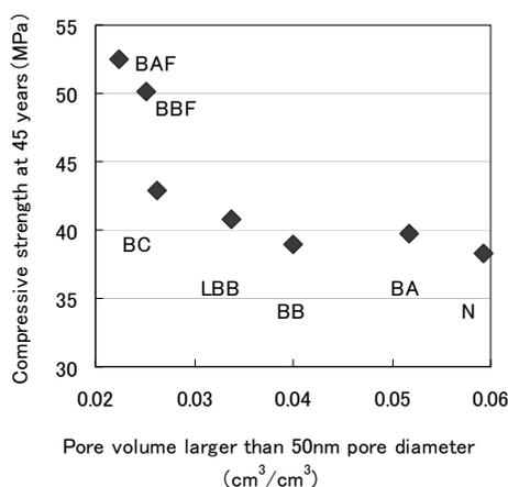
Figure 9. Relationship between pore volume larger than 50-nm pore diameter and compressive strength
