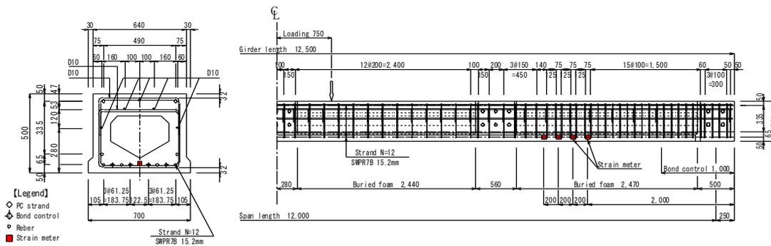
**Figure 4. Details of Girder BS12-EN (Dimension: mm)**
