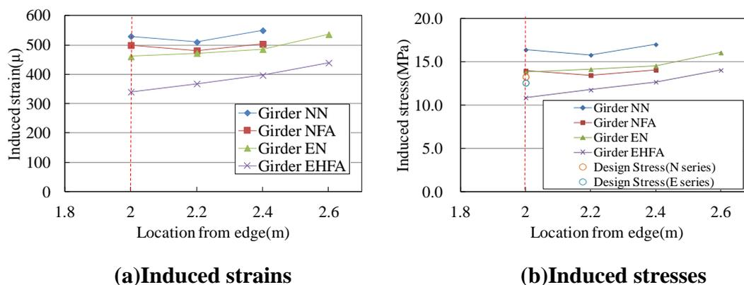
**Figure 5. Induced strains and stresses versus measuring points**
