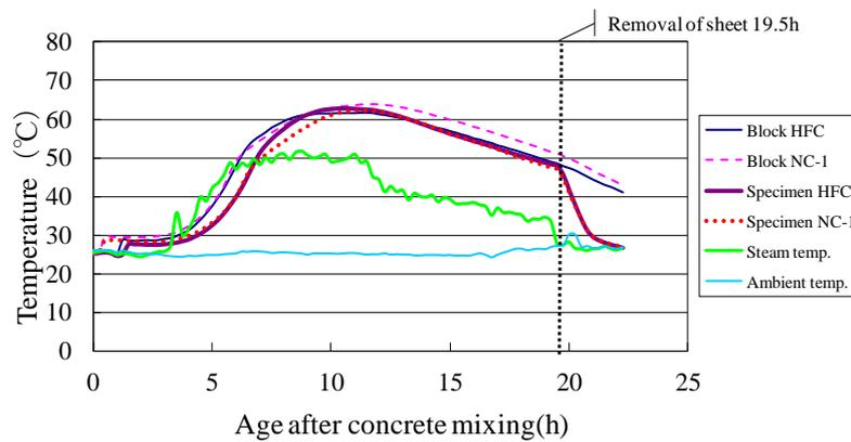
**Figure 2. Temperature histories of NC-1 and HFC cured at 50 °C**
