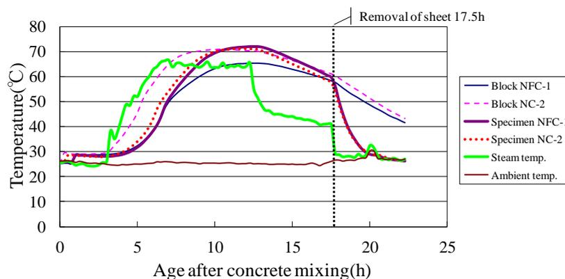
**Figure 3. Temperature histories of NC-2 and NFC-1 cured at 65 °C**
