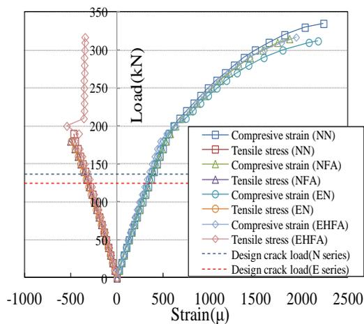
**Figure 6. Loads versus strains**
