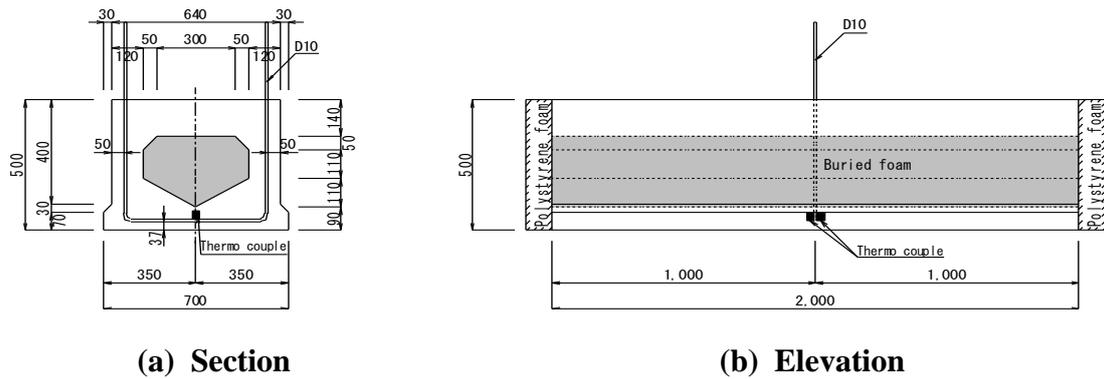
**Figure 1. Details of cross section and elevation (Dimension: mm)**
