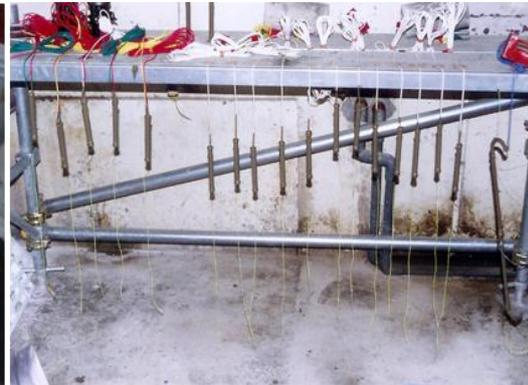
**Figure 4. Drying of steel bars after application of cement paste coating**
