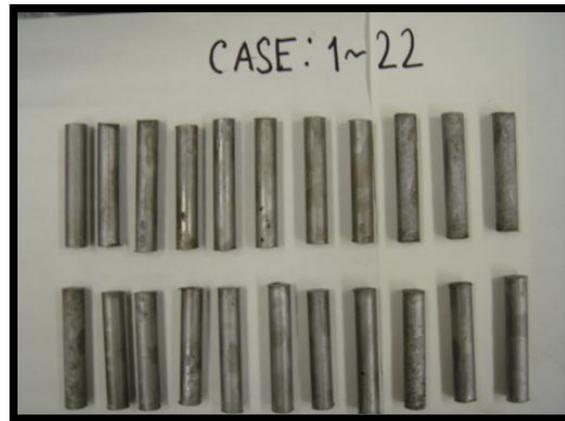
**Figure 16. Visual observation of steel bars after removing the cement paste**
