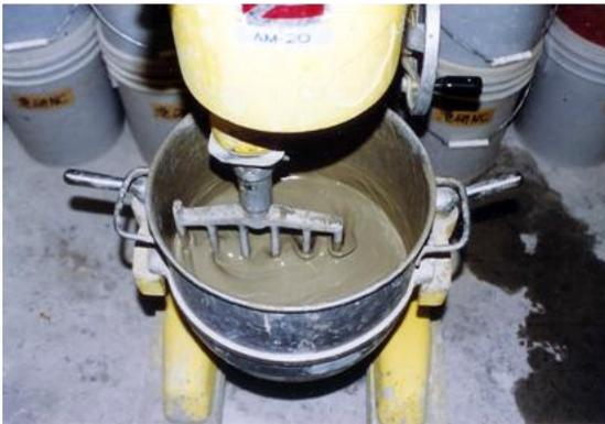
**Figure 3. Mixing of cement paste**
