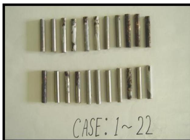
**Figure 15. Visual observation after split the specimen and before removing the paste (45 cycle)**
