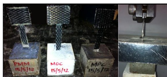
Fig.5. Specimens for pullout test and test setup
