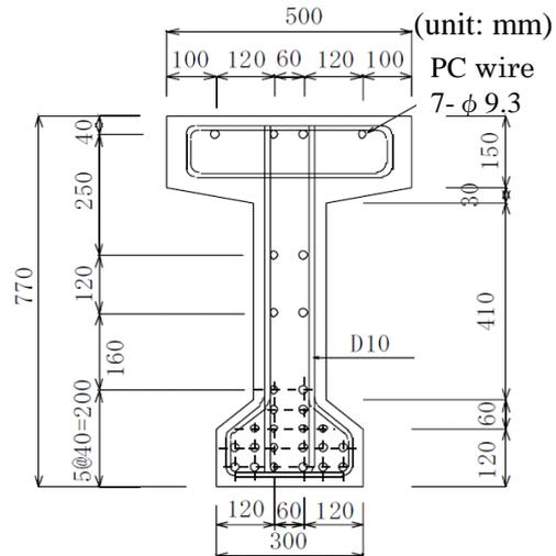
**Figure 2. Cross-Section of PC girder**
