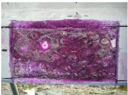
**Photograph 6. Mortar around Anode (TM system : after 10 years)**
