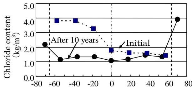
Figure 10. Chloride Content (TG system : over protective)
