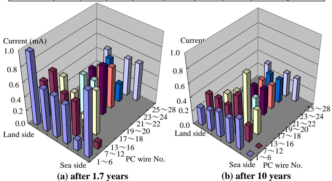
**Figure 11. Supplied Protective Current of Each PC wires (TG system)**
