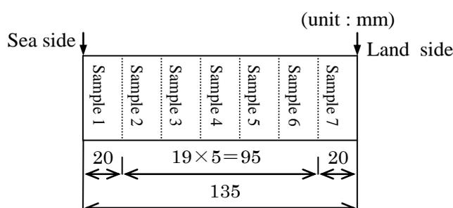
Figure 6. The Cut Position of Core Sample
