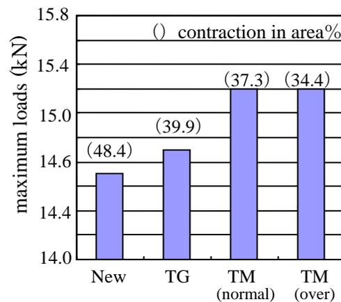
**Figure 13. maximum loads and contraction in area**
