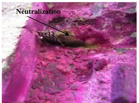
**Photograph 5. Mortar around Anode (TG system : after 10 years)**
