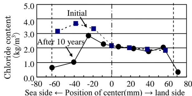
Figure 9. Chloride Content (TG system : normal protective)
