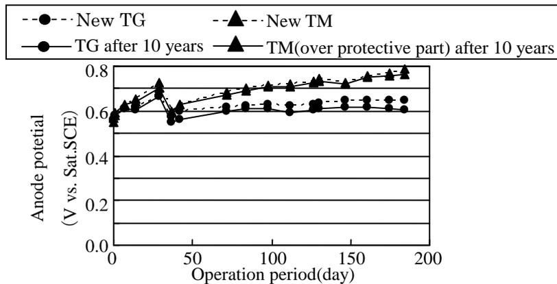
**Figure 12. The result of the accelerated life test(NACE)**
