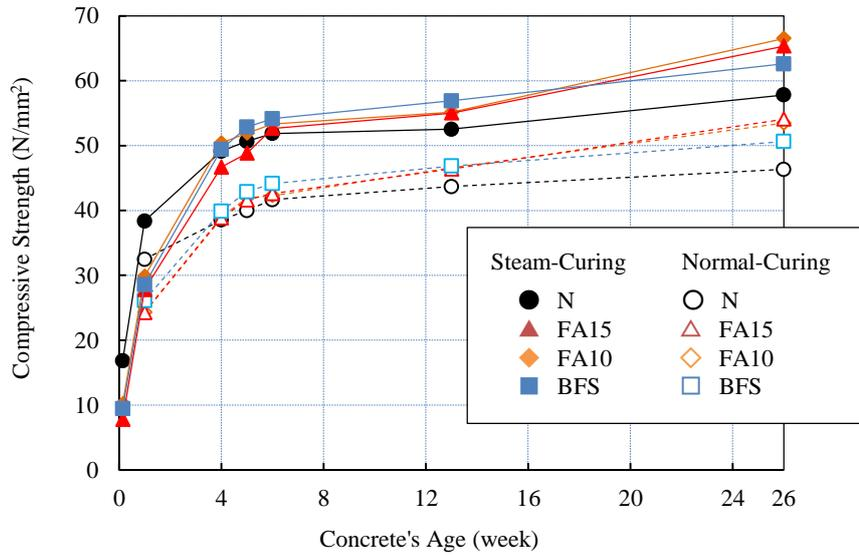
**Fig. 1 Compressive Strength of Concrete**
