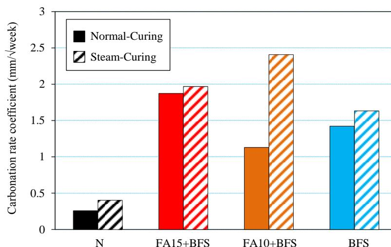
**Fig. 3 Carbonation rate coefficient**
