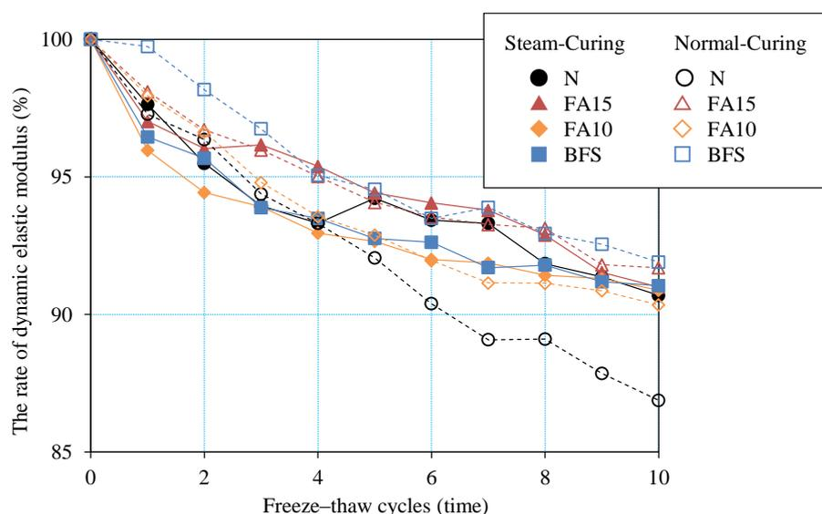
**Fig. 6 The dynamic elastic modulus subjected to freeze–thaw cycles**
