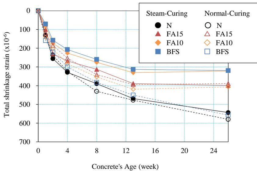
**Fig. 2 Time-dependent change in total shrinkage strain**
