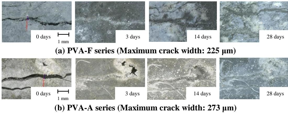
Figure 5. Microscopic observation of precipitation around crack
