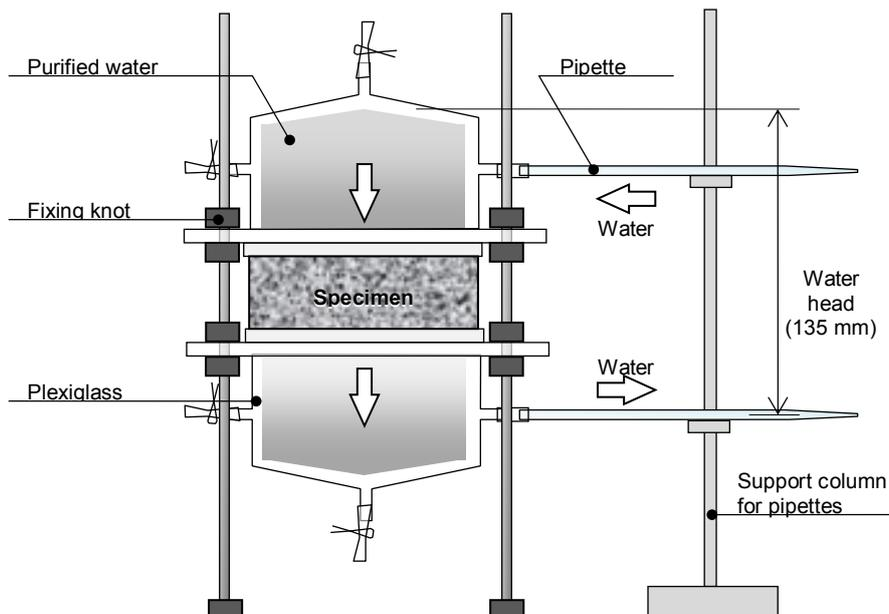
**Figure 2. Apparatus for water permeability test**
