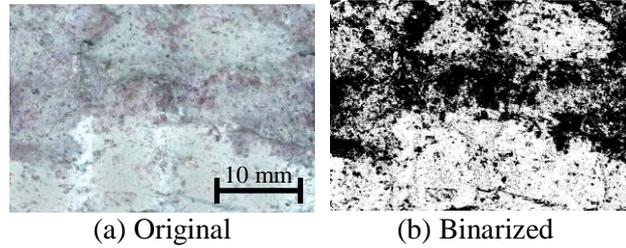
**Figure 3. Calculation of precipitated area**
