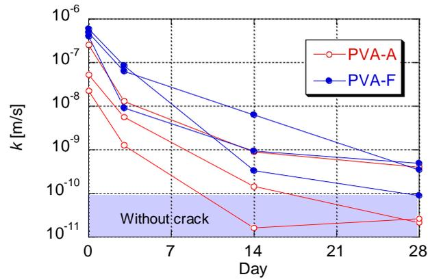
Figure 6. Relationship between time and coefficient of water permeability ( $k$ )
