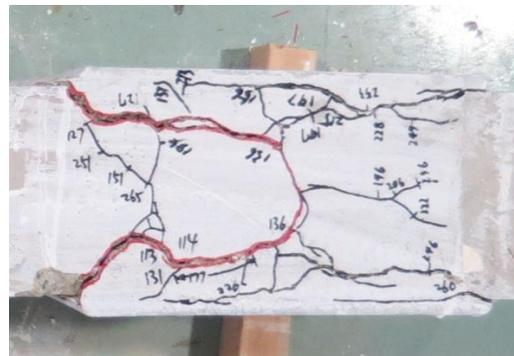
**Figure 12. Cracks on the bottom of U1.5**
