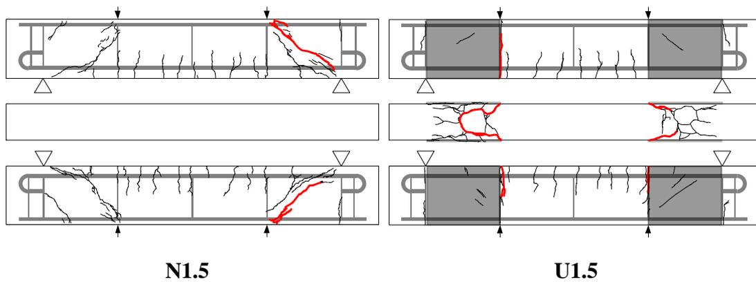
**Figure 11. Crack condition (Group 2)**
