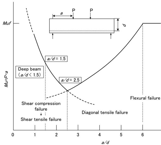
**Figure 1. Conceptual figure of the relationship between shear-span ratio and failure mode**
