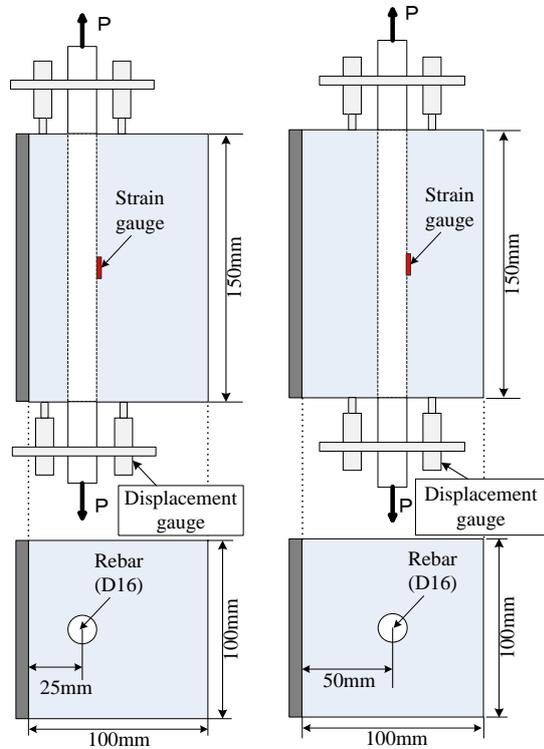
**Figure 4. Dimensions of test blocks**
