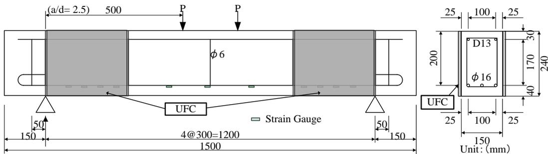
**Figure 2. Dimensions of RC beams and Locations of UFC panel (Group 1)**
