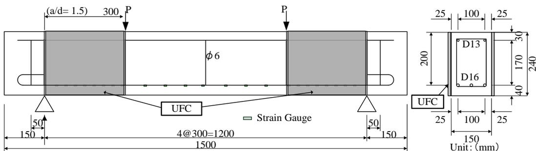
**Figure 3. Dimensions of RC beams and Locations of UFC panel (Group 2)**
