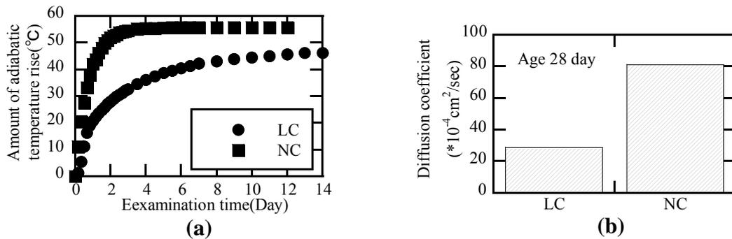
Figure 3. (a) Adiabatic temperature rise and (b) Diffusion coefficient.
