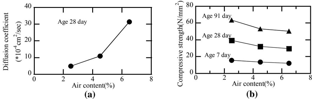
**Figure 6. (a) Diffusion coefficient and (b) Compressive strength**
