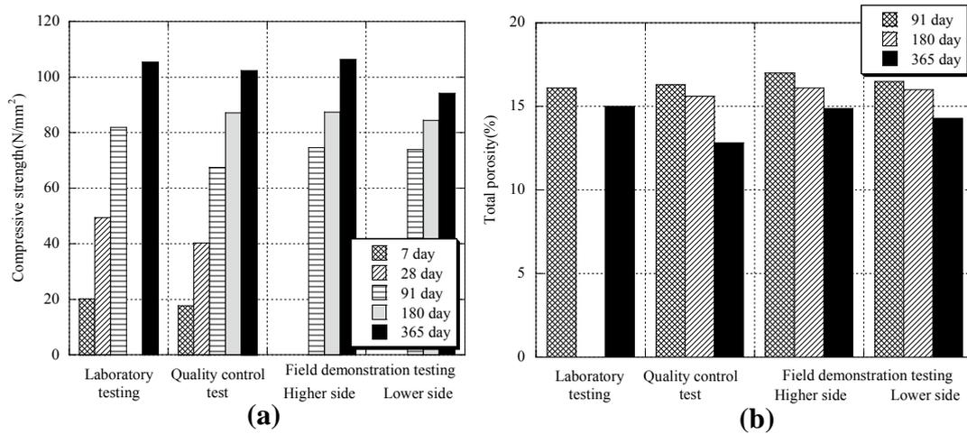
Figure 10 (a) Compressive strength and (b) total porosity
