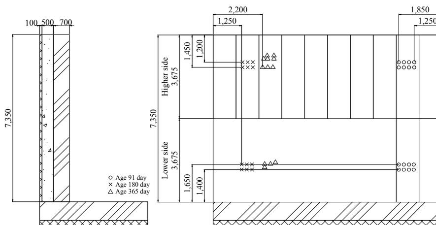
**Figure 9 Core sampling positions**
