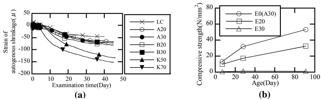
Figure 4. (a) Autogenous shrinkage and (b) Compressive strength
