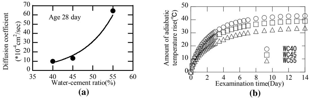
**Figure 5. (a) Diffusion coefficient and (b) Adiabatic temperature rise**
