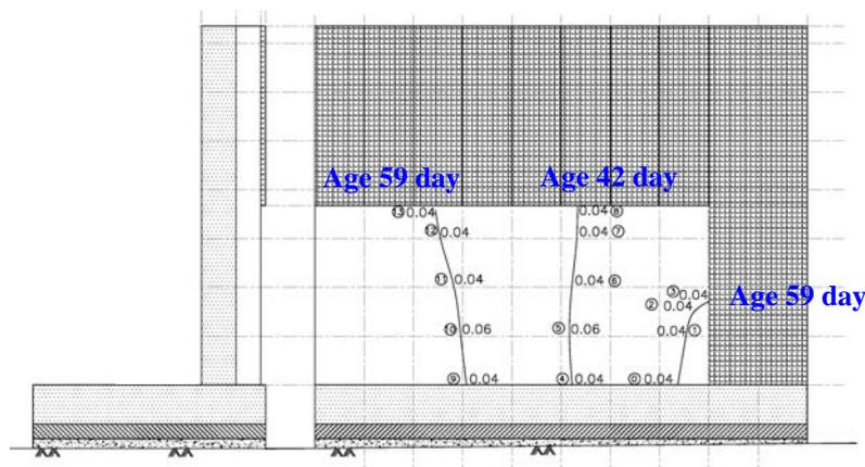
**Figure 12 Crack generating situation**
