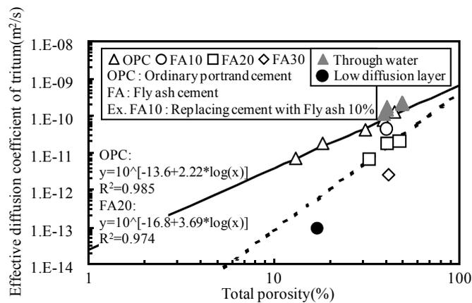
Figure 11 Total porosity and effective diffusion coefficient of tritium
