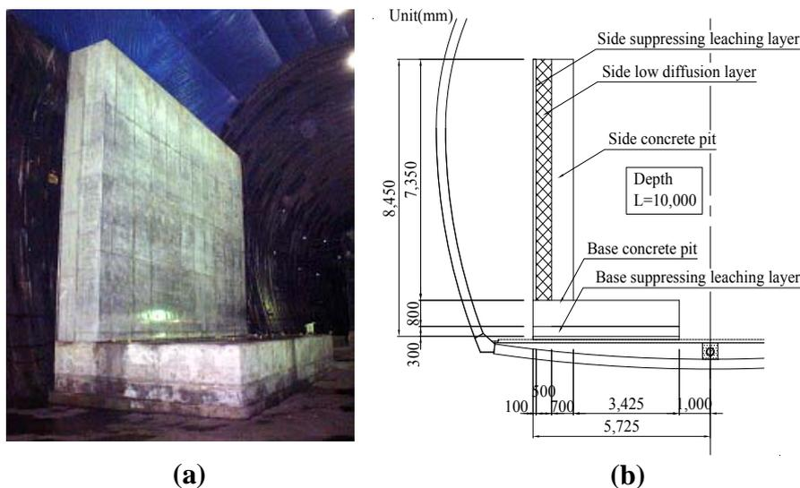
**Figure 8 Full-size model (a) Overview, (b) Cross section**
