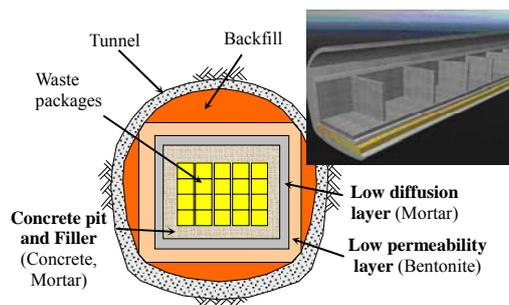
**Figure 1. Sub-surface disposal facility**
