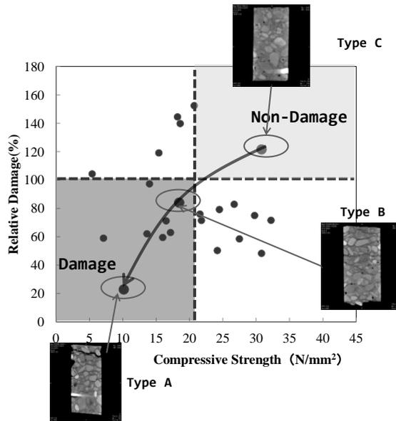
**Figure 7. Comparison of relative damage and compressive strength.**
