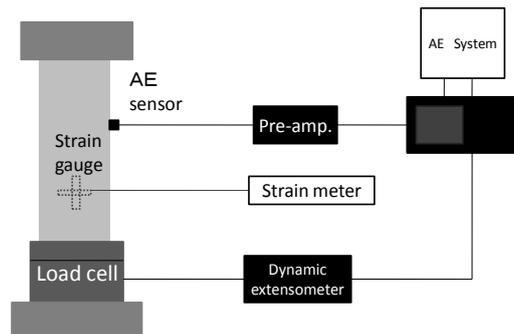
**Figure 4. Test setup for AE in core test.**
