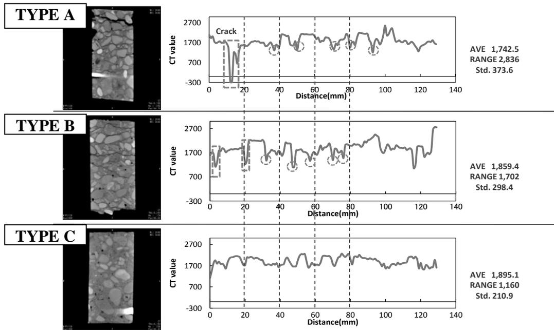
Figure 5. Results of X-ray density analysis from top to bottom in core-sample.
