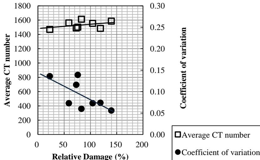
**Figure 8. Comparison of relative damage and statistical properties of CT data.**
